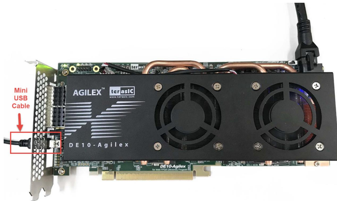
Figure 10-2 Connection setup for using dashboard system
