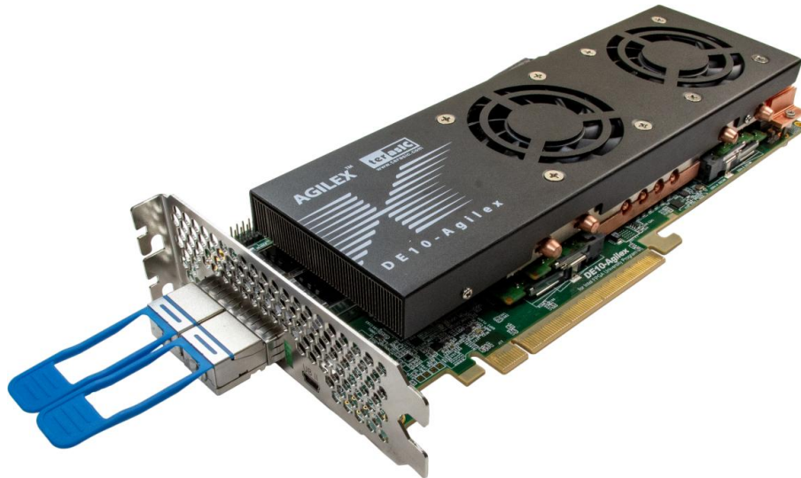
Figure 9-2 QSFP-DD Transceiver Loopback Test in Progress
