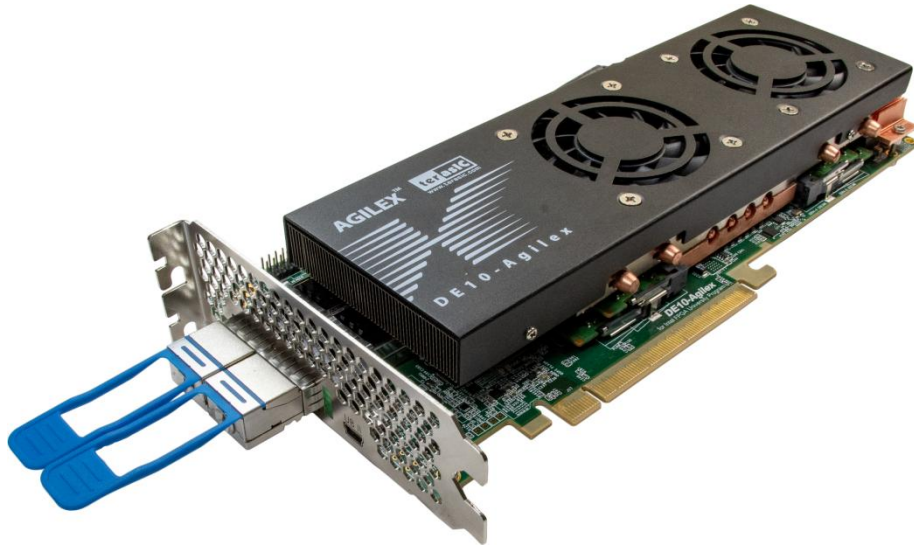
Figure 9-14 Setup QSFP28 or QSFPDD loopback fixture
