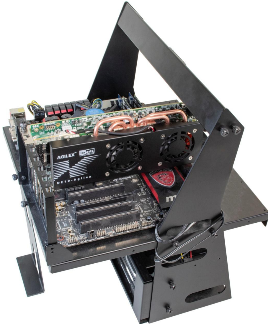
Figure 7-9 FPGA board installation on PC
