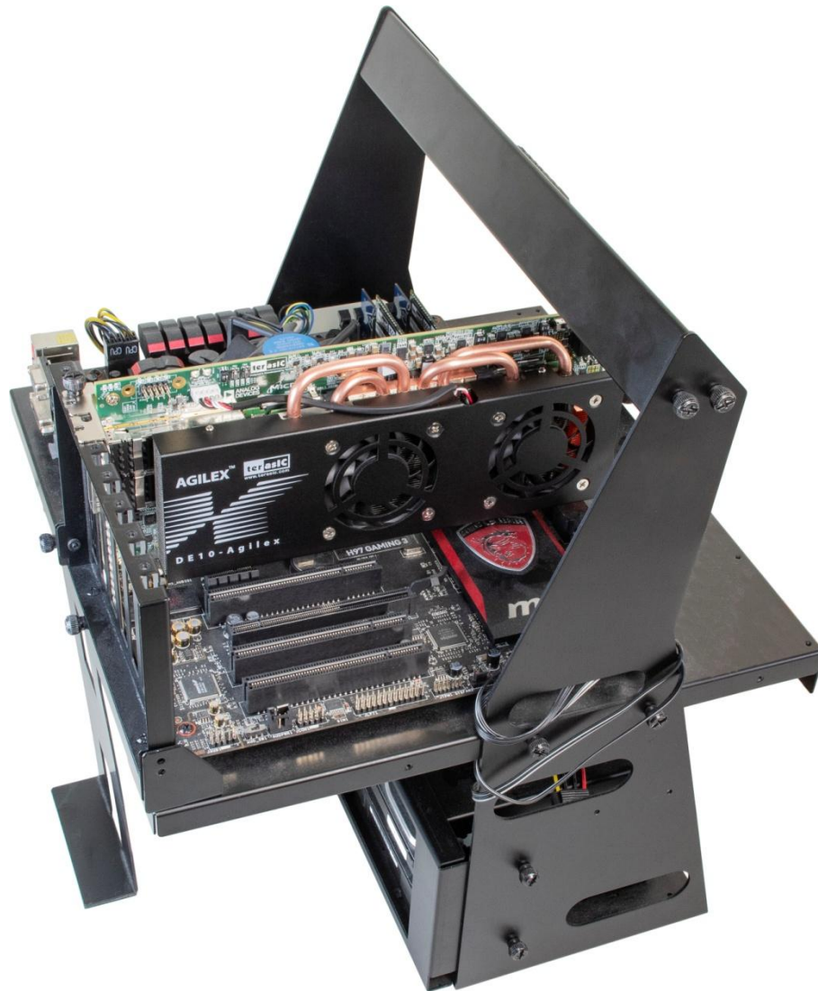
Figure 8-4 FPGA board installation on PC
