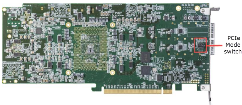
Figure 2-7 Position of the PCIe mode switch
