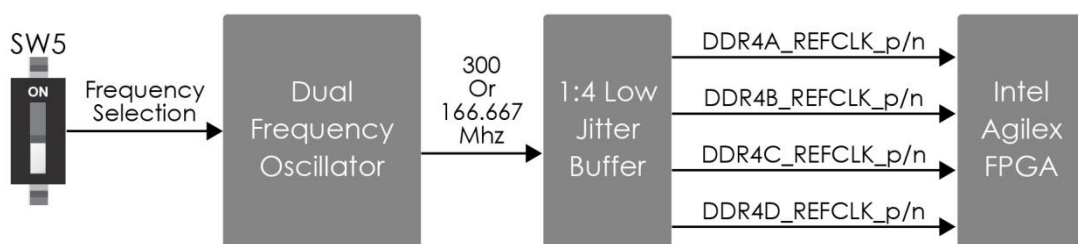
Figure 2-11 The DDR4 reference clock diagram
