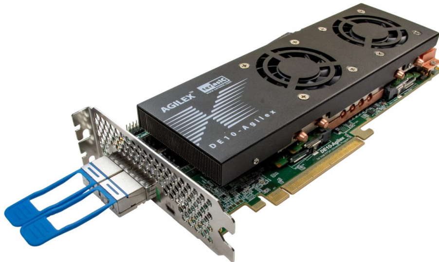
Figure 9-2 QSPF-DD Transceiver Loopback Test in Progress
