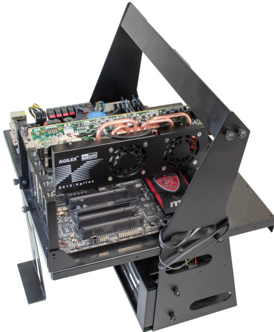
Figure 8-4 FPGA board installation on PC
