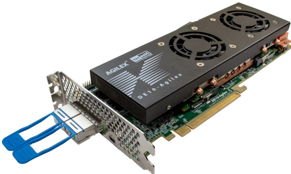
Figure 9-9 Setup QSFP28 or QSFPDD loopback fixture
