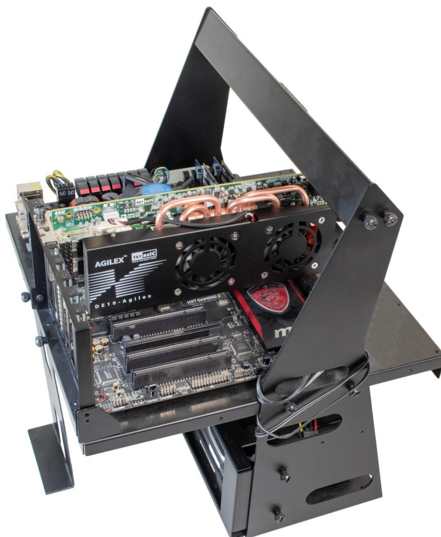
Figure 7-9 FPGA board installation on PC
