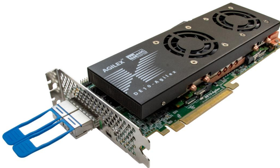
Figure 9-14 Setup QSFP28 or QSFPDD loopback fixture
