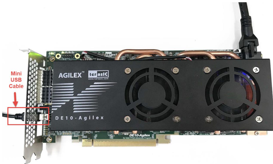
Figure 10-2 Connection setup for using dashboard system
