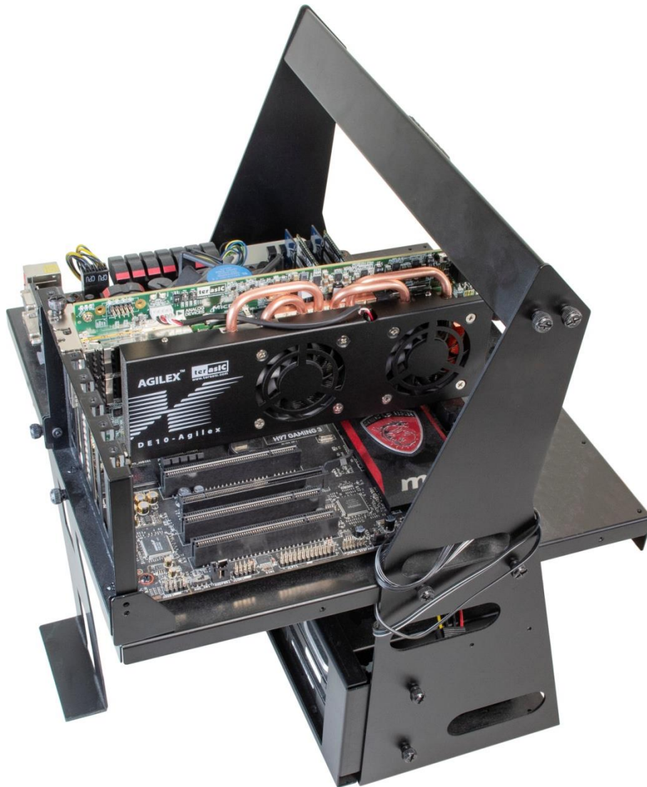
Figure 8-4 FPGA board installation on PC
