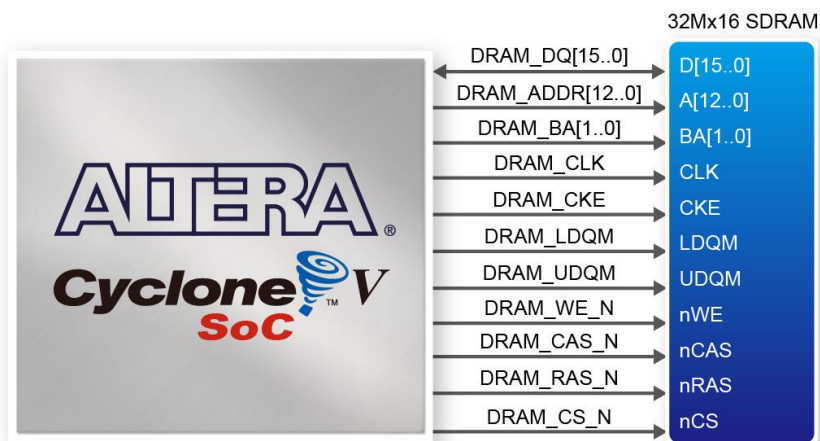
Figure 3-28 Connections between the FPGA and SDRAM
