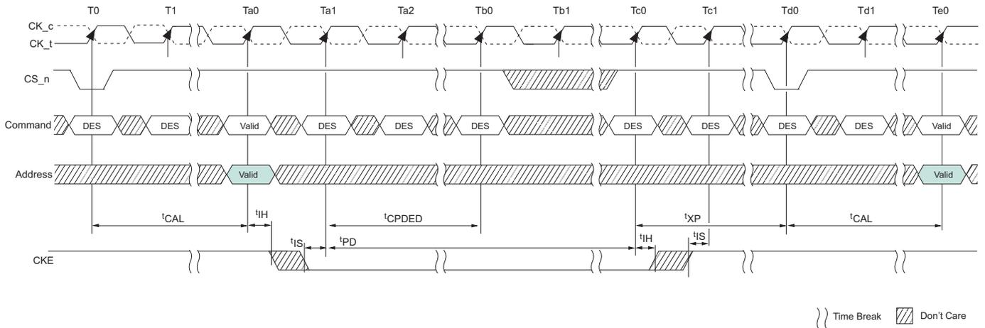
**Figure 104: REFRESH Command to Power-Down Entry with CAL**
