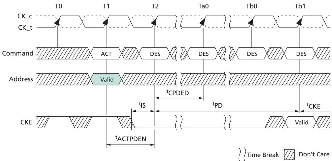
Figure 100: PRECHARGE/PRECHARGE ALL Command to Power-Down Entry
