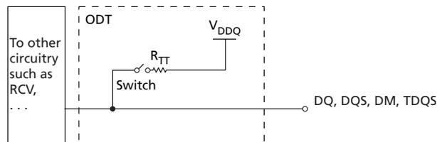
The switch is enabled by the internal ODT control logic, which uses the external ODT pin and other control information. The value of  $R_{TT}$  is determined by the settings of mode register bits (see Mode Register). The ODT pin will be ignored if the mode register MR1 is programmed to disable  $R_{TT(NOM)}$  [MR1[10,9,8] = 0,0,0] and in self refresh mode.
