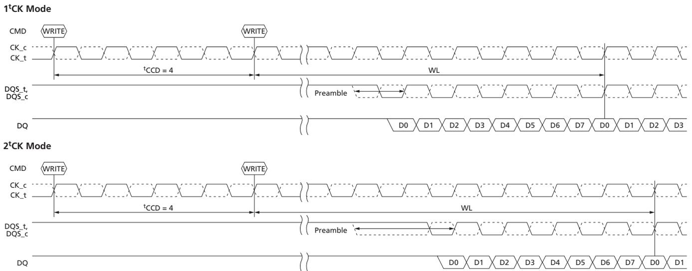
**Figure 112: 1<sup>t</sup>CK vs. 2<sup>t</sup>CK WRITE Preamble Mode, t<sub>CCD</sub> = 5**
