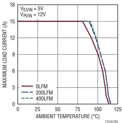
**Figure 3. Current Derating at 500kHz, 5V<sub>SVIN</sub>**
