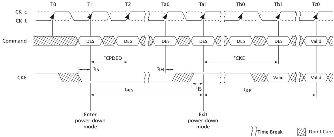
Figure 98: REFRESH Command to Power-Down Entry
