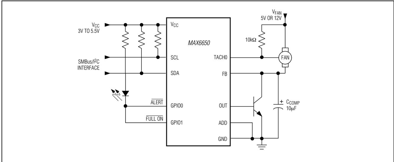
Figure 6. Fan Control with a Bipolar Transistor
