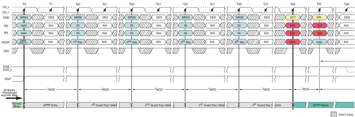
Figure 79: sPPR – Repair, and Exit
