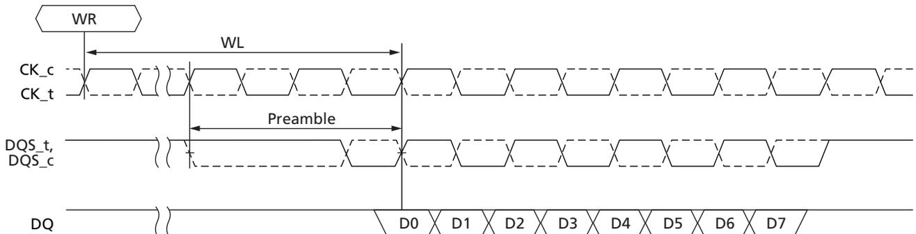
CWL has special considerations when in the 2<sup>t</sup>CK WRITE preamble mode. The CWL value selected in MR2[5:3], as seen in table below, requires at least one additional clock when the primary CWL value and 2<sup>t</sup>CK WRITE preamble mode are used; no additional clocks are required when the alternate CWL value and 2<sup>t</sup>CK WRITE preamble mode are used.
