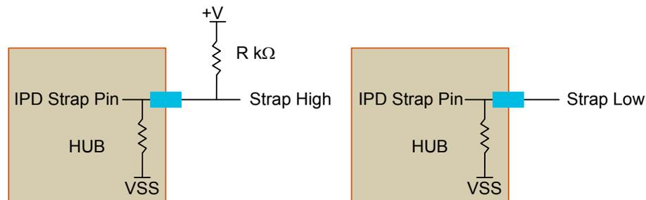
**Figure 3.5 Pin Strap Option with IPD Pin Example**
