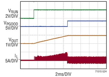
$V_{IN} = 12\text{V}$ ,  $C_{TRACK/SS} = 0.1\mu\text{F}$
