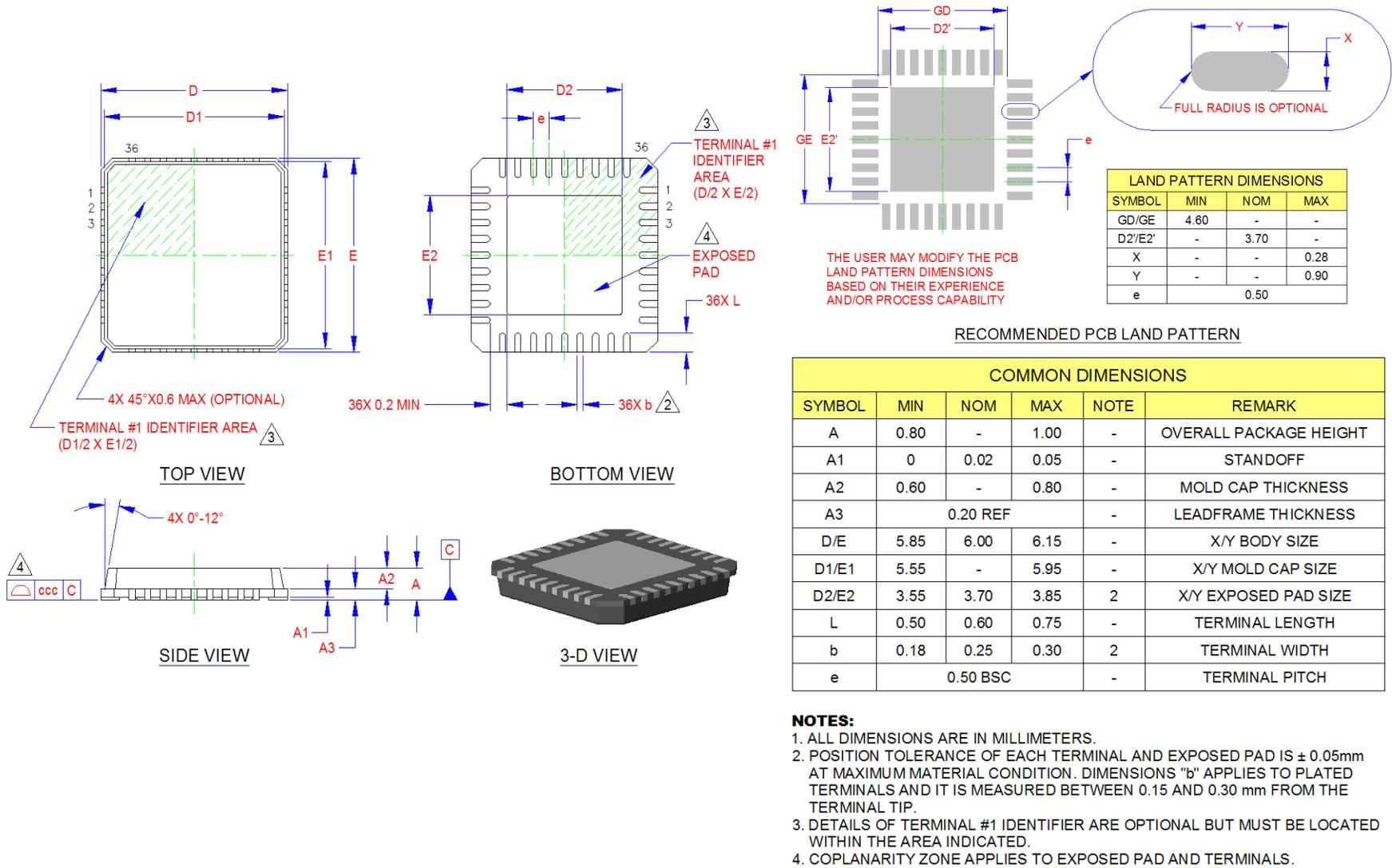
Figure 8.1 36-Pin QFN, 6x6 mm Body, 0.5 mm Pitch
