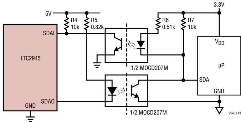
Figure 13. Opto-Isolation of a 10kHz I<sup>2</sup>C Interface Between LTC2945 and Microcontroller (SCL Omitted for Clarity)
