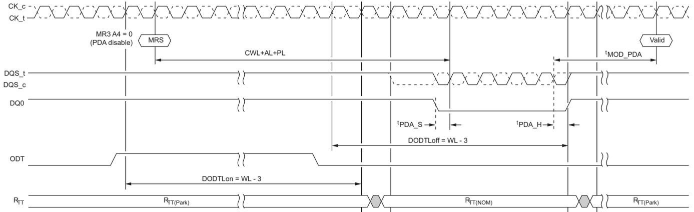
Note: 1. R<sub>TT</sub>(Park) = Enable; R<sub>TT</sub>(NOM) = Enable; WRITE preamble set = 2<sup>t</sup>CK; and DLL = On.
