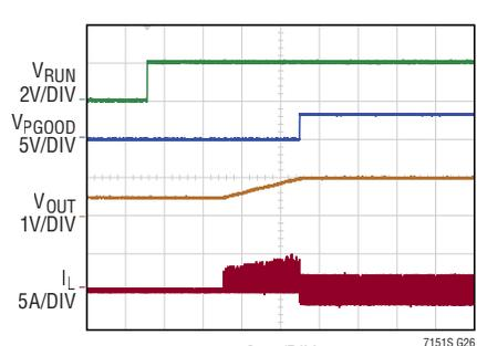
$V_{IN} = 12\text{V}$ ,  $C_{TRACK/SS} = 0.1\mu\text{F}$
