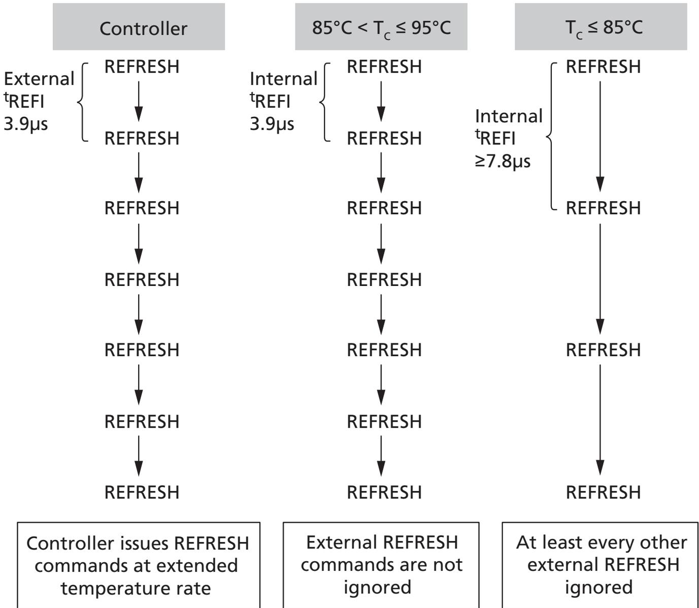
Note: 1. TCR enabled with Extended Temperature Mode selected.
