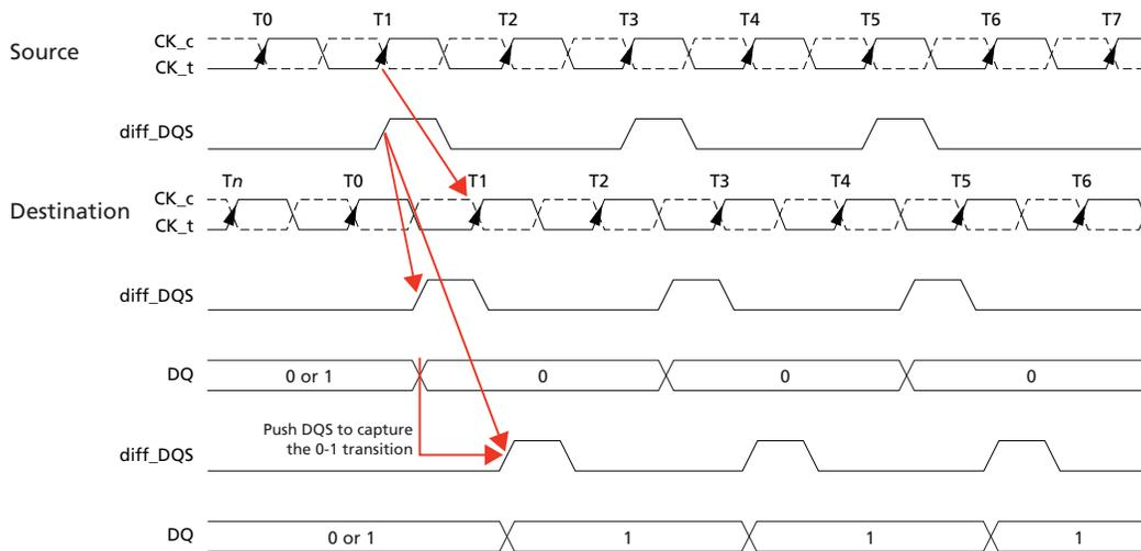
DQS driven by the controller during leveling mode must be terminated by the DRAM based on the ranks populated. Similarly, the DQ bus driven by the DRAM must also be terminated at the controller.
