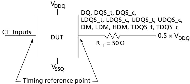
**Figure 235: Connectivity Test Mode Output Slew Rate Definition**
