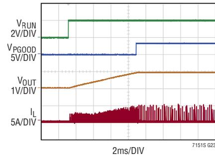
$V_{IN} = 12\text{V}$ ,  $C_{TRACK/SS} = 0.1\mu\text{F}$
