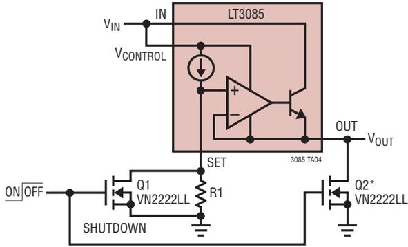
\*Q2 INSURES ZERO OUTPUT IN THE ABSENCE OF ANY OUTPUT LOAD.
