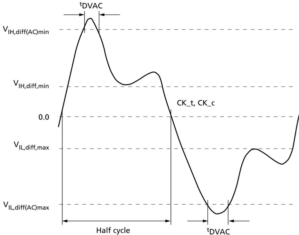
Notes: 1. Differential signal rising edge from  $V_{IL,diff,max}$  to  $V_{IH,diff(AC)min}$  must be monotonic slope.
