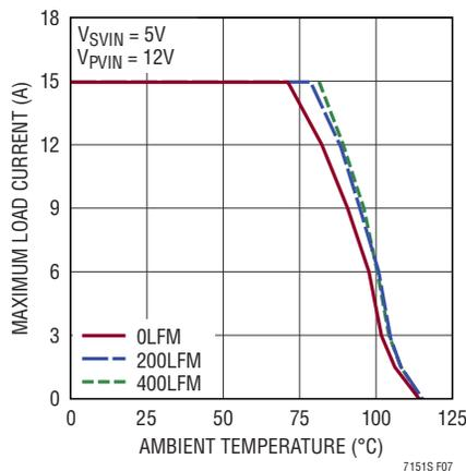
**Figure 7. Current Derating at 2MHz, 5V<sub>SVIN</sub>**
