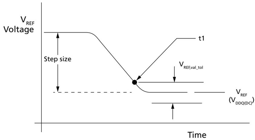
**Figure 70: V<sub>REF</sub> Full Step: From V<sub>REF,min</sub> to V<sub>REF,max</sub> Case**
