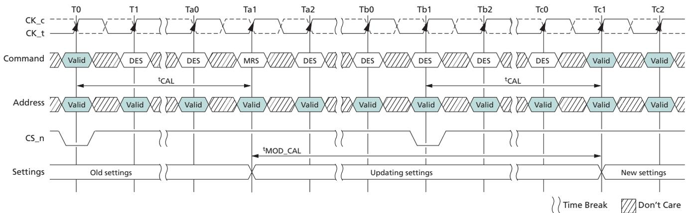
Note: 1. MRS at Ta1 may or may not modify CAL,  $t_{MOD\_CAL}$  is computed based on new  $t_{CAL}$  setting if modified.
