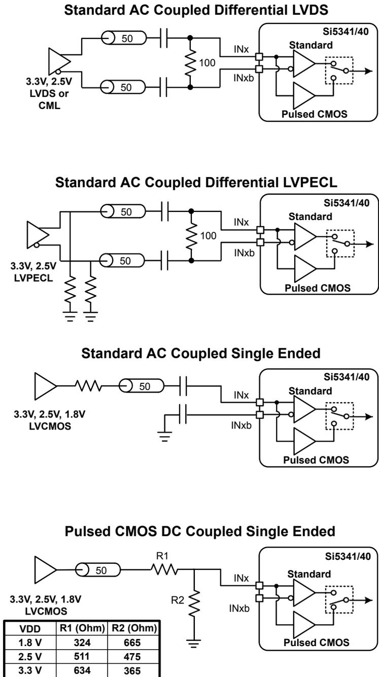
**Figure 3.3. Termination of Differential and LVCMOS Input Signals**
