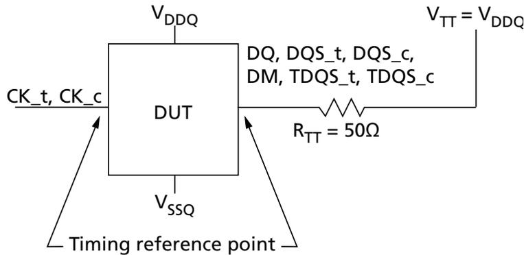
**Connectivity Test Mode Output Levels**
