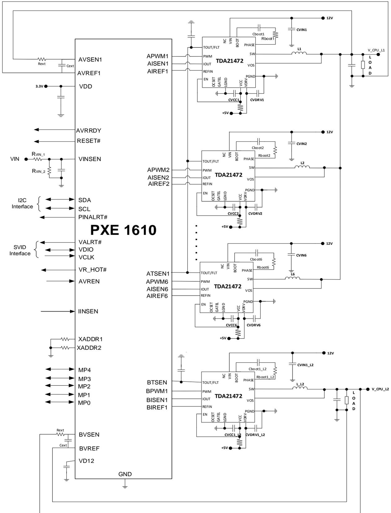
Figure 11 6+1 - Phase Voltage Regulator - Typical Application (simplified schematic)
