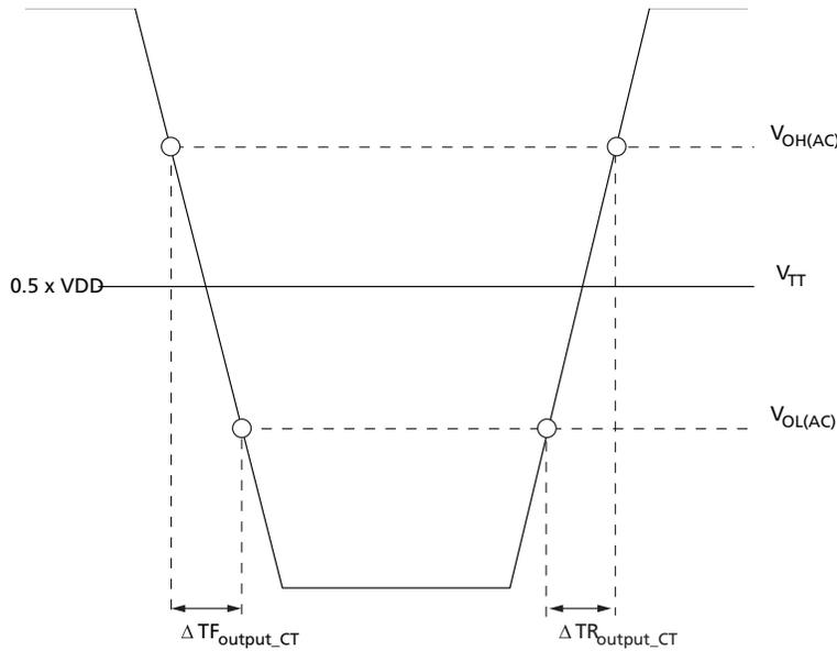
**Table 121: Connectivity Test Mode Output Slew Rate**
