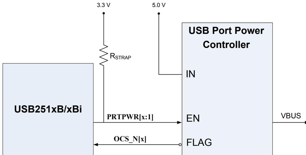
Figure 4.1 Battery Charging via External Power Supply
