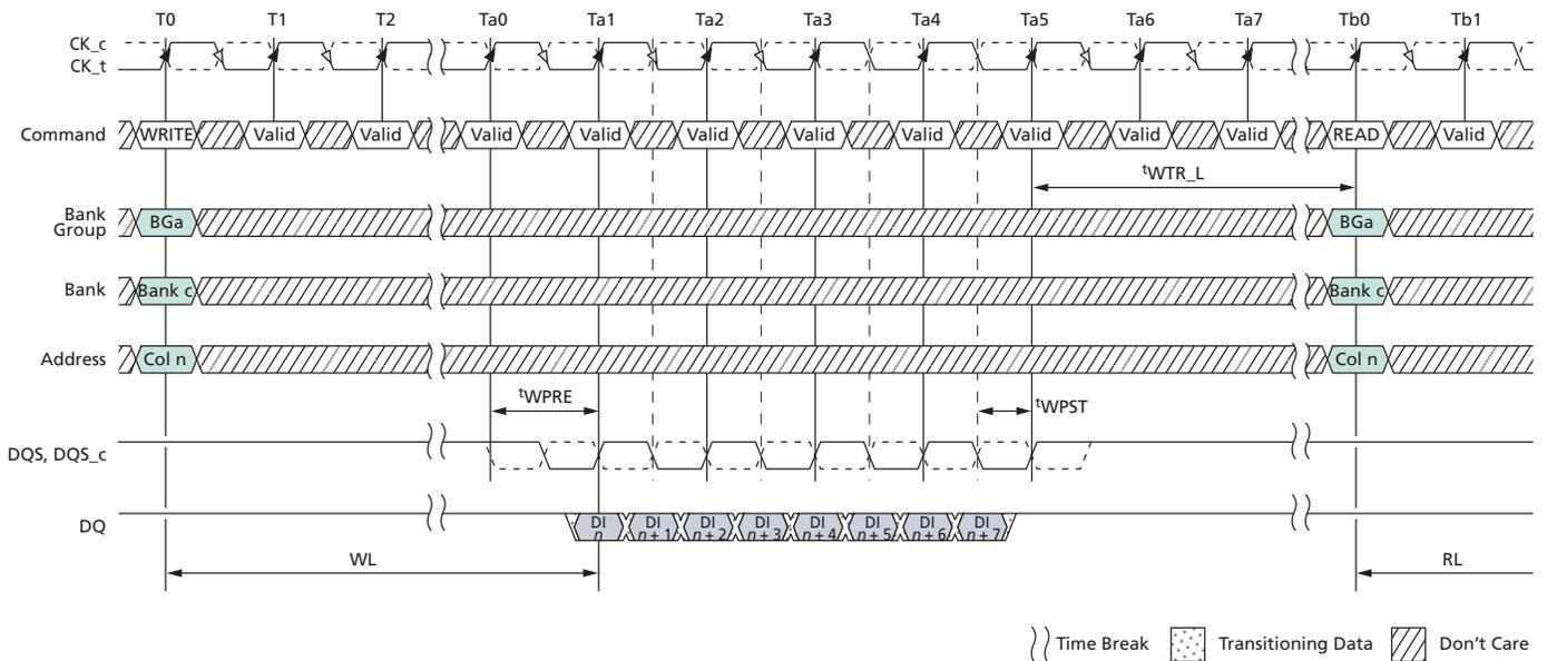
Note: 1.  $t^{\text{WTR\_L}}$ : delay from start of internal write transaction to internal READ command to the same bank group.
