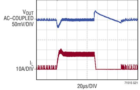
$V_{IN} = 12\text{V}$ ,  $V_{OUT} = 1\text{V}$
