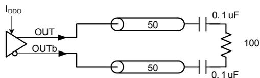
**LVCMOS Output Test Configuration**
