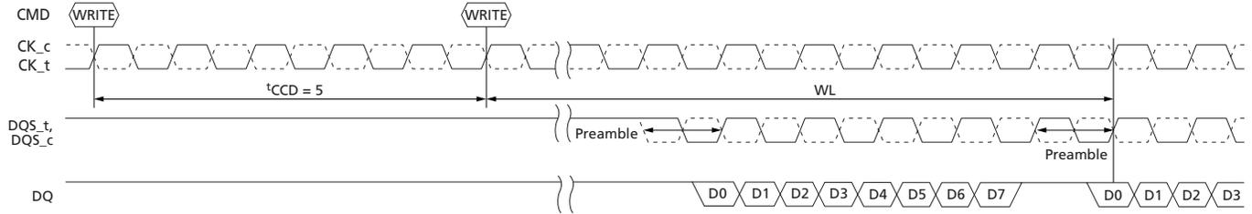
**2<sup>t</sup>CK Mode:** t<sub>CCD</sub> = 5 is not allowed in 2<sup>t</sup>CK mode.
