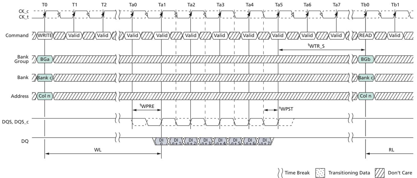
Note: 1.  $t^{\text{WTR\_S}}$ : delay from start of internal write transaction to internal READ command to a different bank group.
