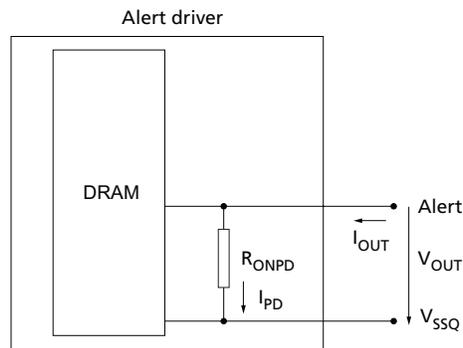
$R_{ONPD}$  when  $R_{ONPU}$  is off:
