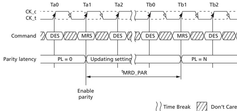
Note: 1.  $t_{MRD\_PAR} = t_{MOD} + N$ ; where N is the programmed parity latency.
