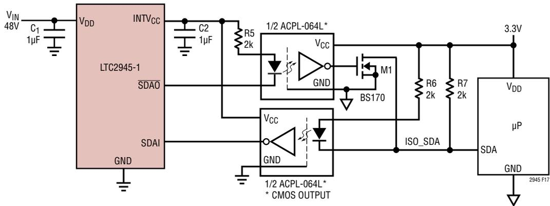
Figure 17. Opto-Isolation of I<sup>2</sup>C Interface with Low Power, High Speed Opto-couplers (SCL Omitted for Clarity)
