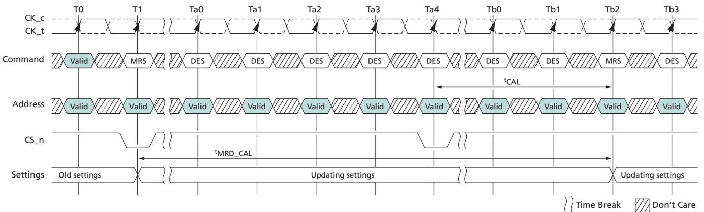
Note: 1. Command address latency mode is enabled at T1.
