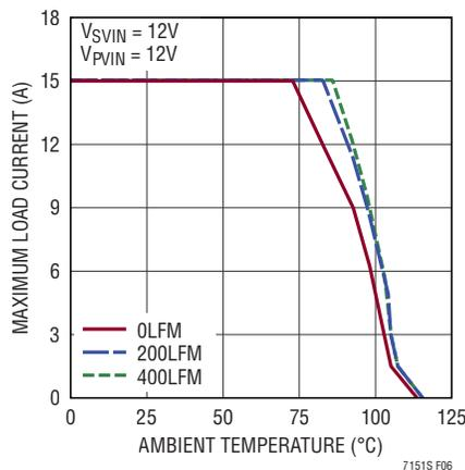
**Figure 6. Current Derating at 1MHz, 12V<sub>SVIN</sub>**
