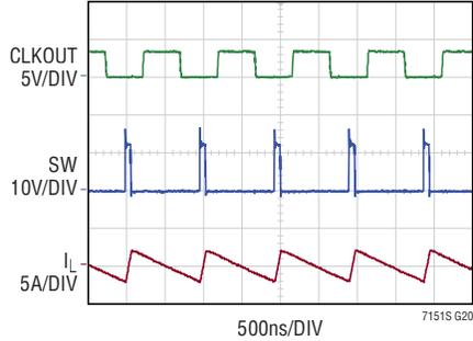
$V_{IN} = 12\text{V}$ ,  $V_{OUT} = 1\text{V}$
