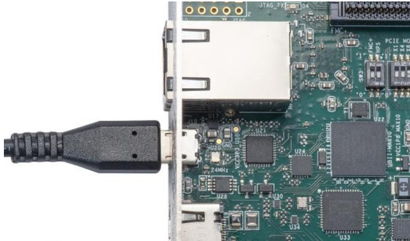
Figure 1-6 Connect the Micro USB cable to the board
