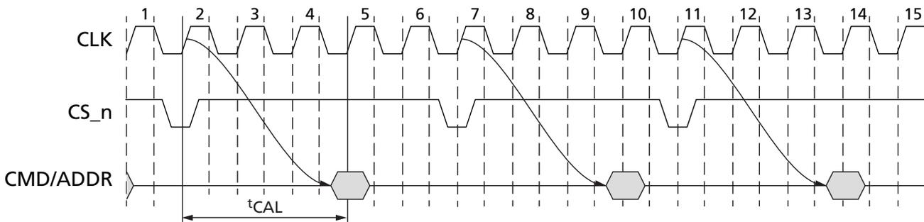
CAL gives the DRAM time to enable the command and address receivers before a command is issued. After the command and the address are latched, the receivers can be disabled if CS<sub>n</sub> returns to HIGH. For consecutive commands, the DRAM will keep the command and address input receivers enabled for the duration of the command sequence.
