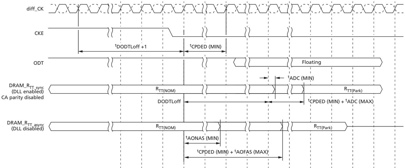
**Figure 106: ODT Power-Down Exit with ODT Buffer Disable Mode**
