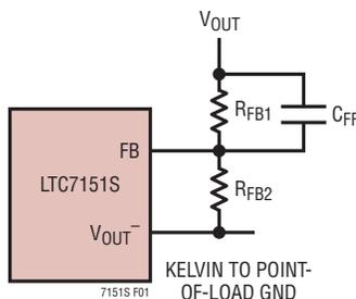
Figure 1. Setting the Output Voltage Differentially
