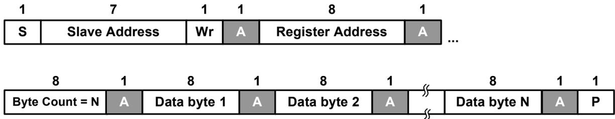
Figure 5.1 Block Write
