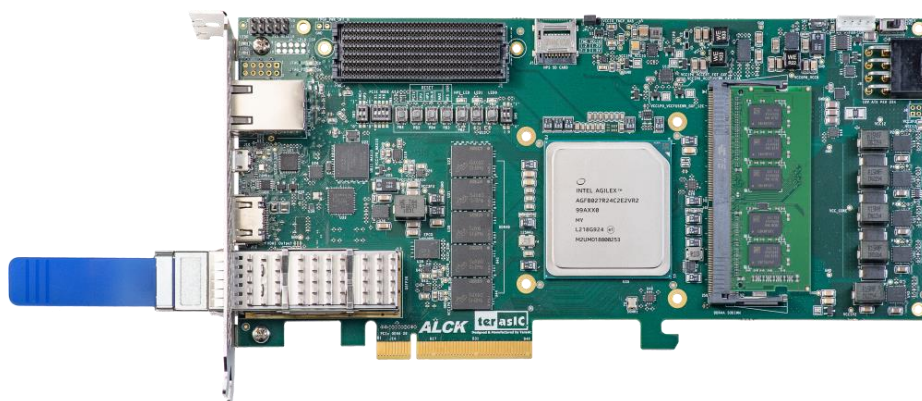
Figure 2-14 Setup QSFP28 loopback fixture
