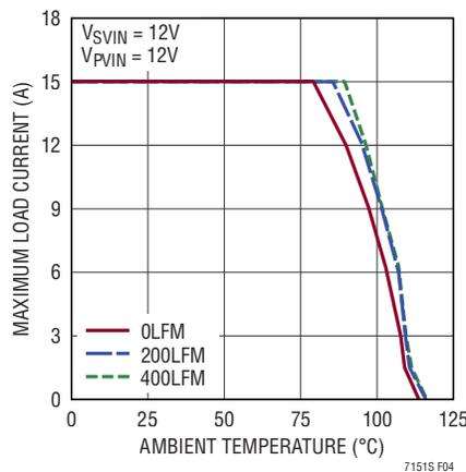
**Figure 4. Current Derating at 500kHz, 12V<sub>SVIN</sub>**
