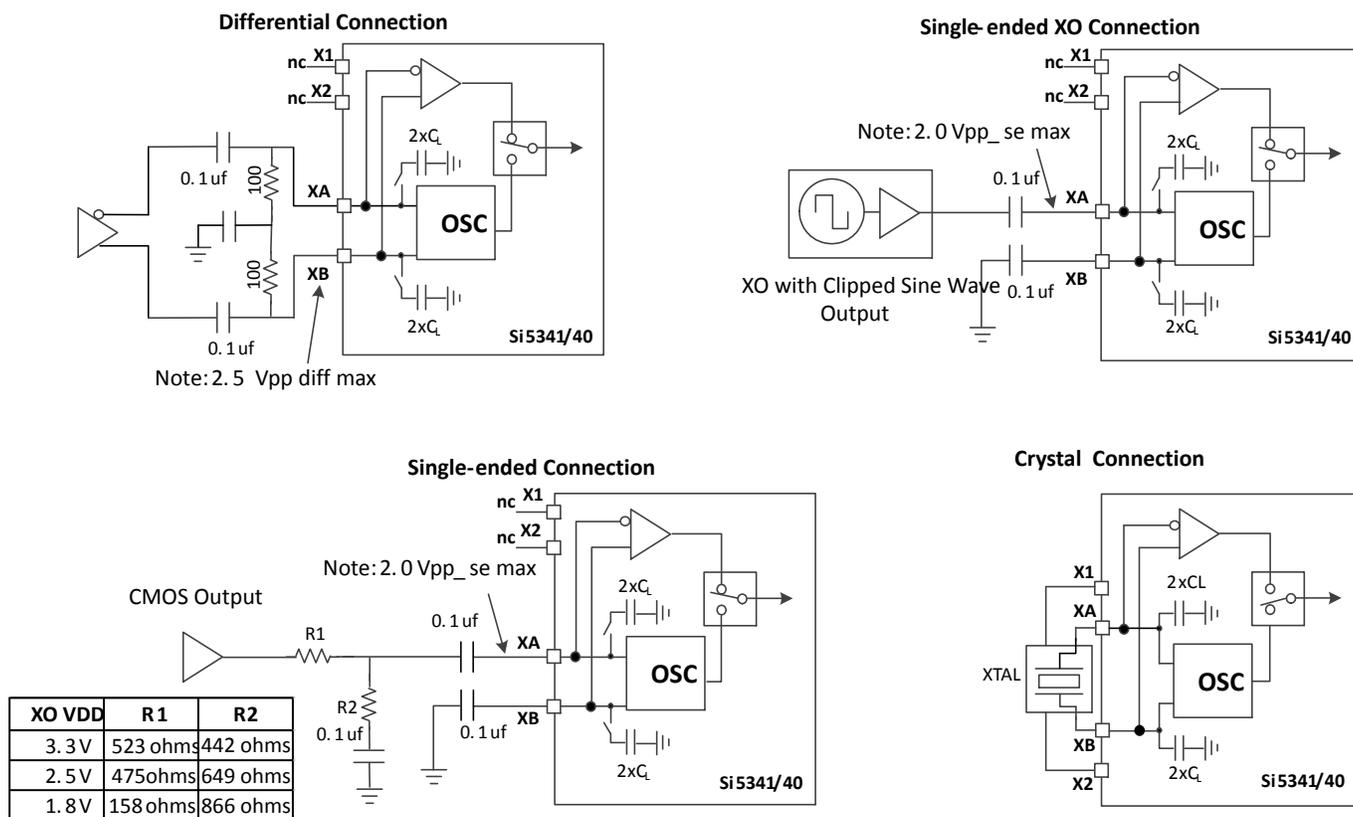
Figure 3.2. XAXB External Crystal and Clock Connections
