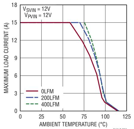
**Figure 8. Current Derating at 2MHz, 12V<sub>SVIN</sub>**
