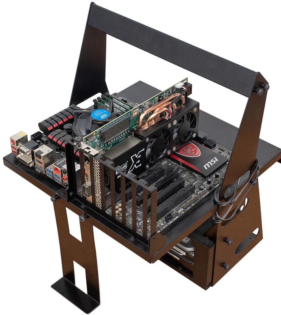
Figure 5-4 FPGA board installation on PC
