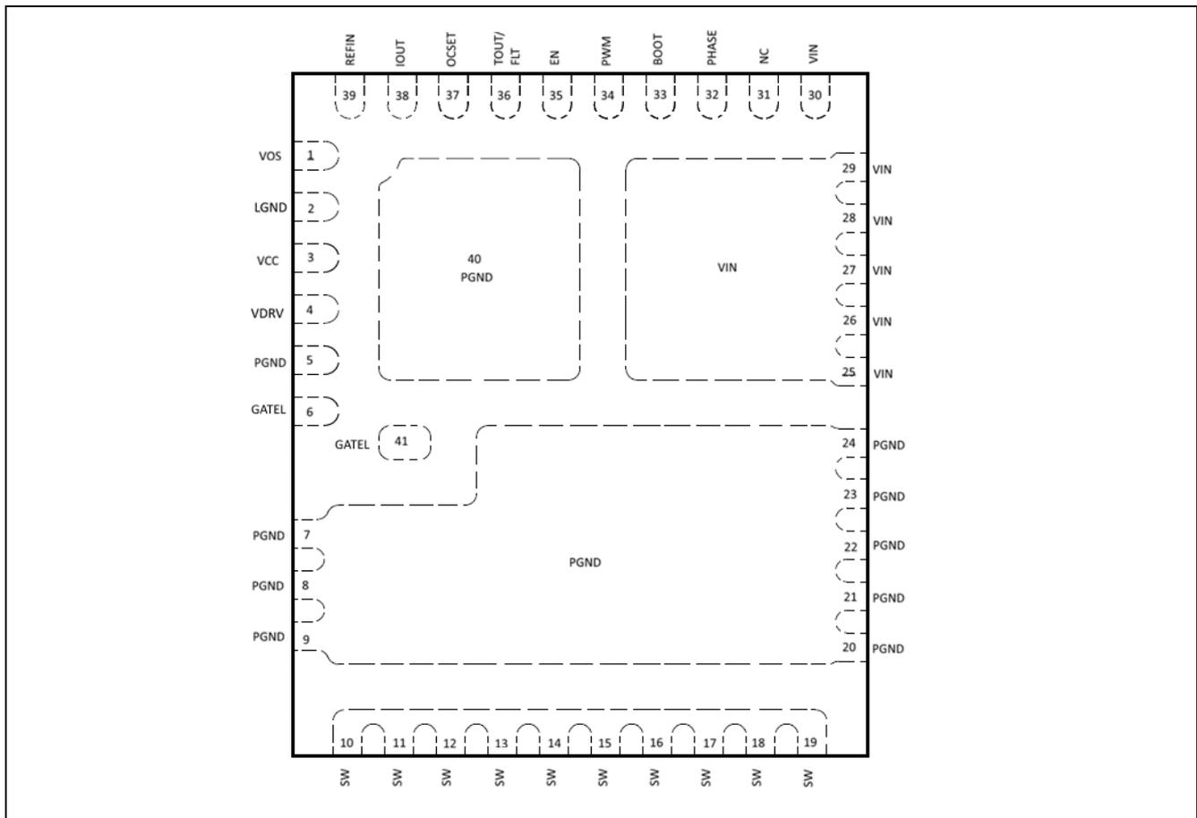
Figure 2 Pinout, Numbering and Name of Pins (transparent top view)
