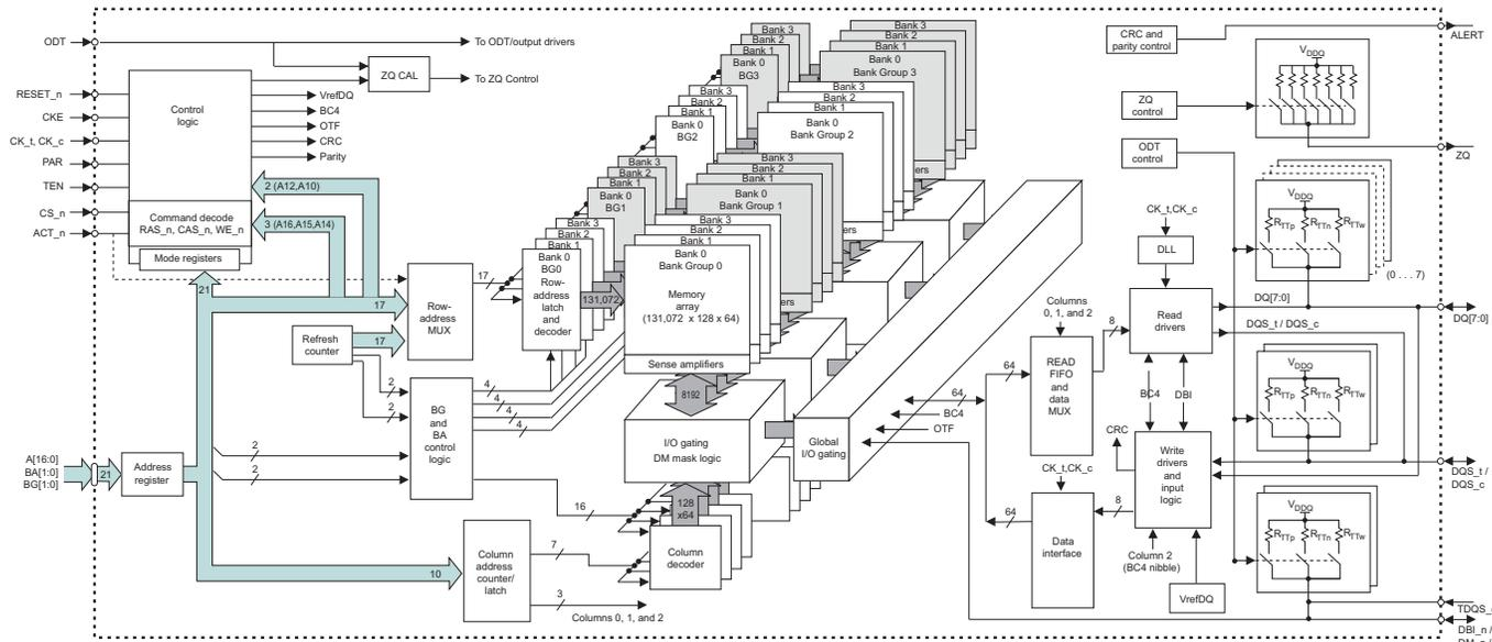
**Figure 4: 1 Gig x 16 Functional Block Diagram**
