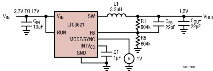
**1.2V<sub>OUT</sub>, Synchronized to 600kHz, Forced Continuous Mode**
