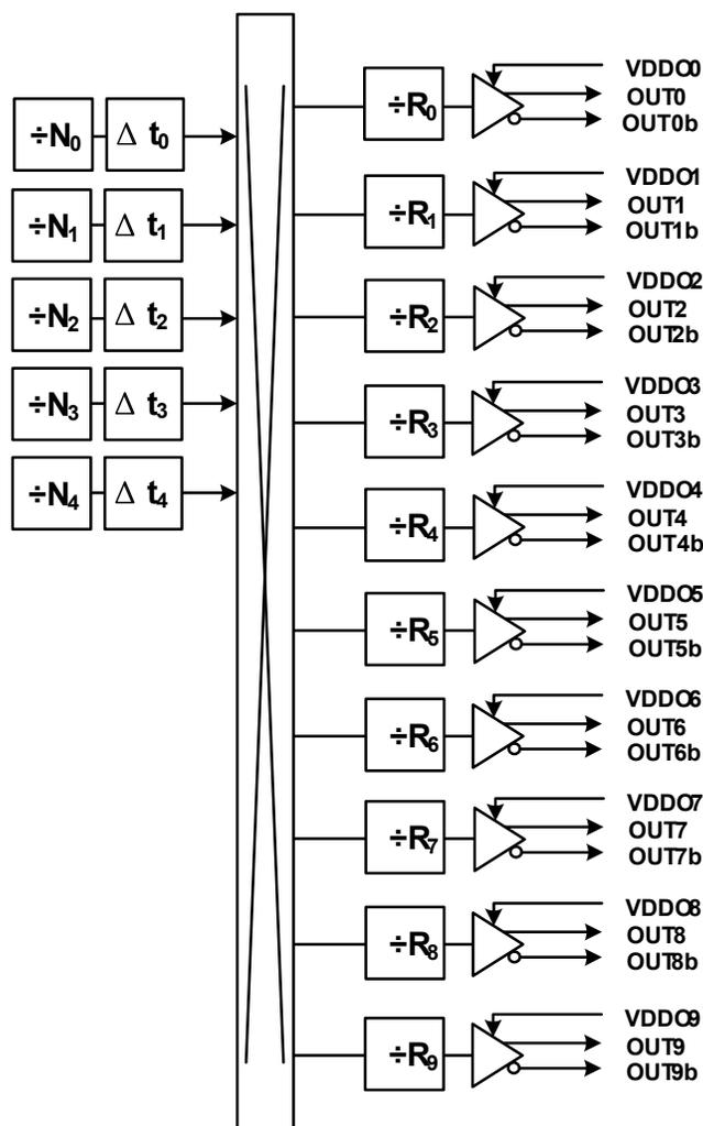
Figure 3.7. Example of Independently Configurable Path Delays
