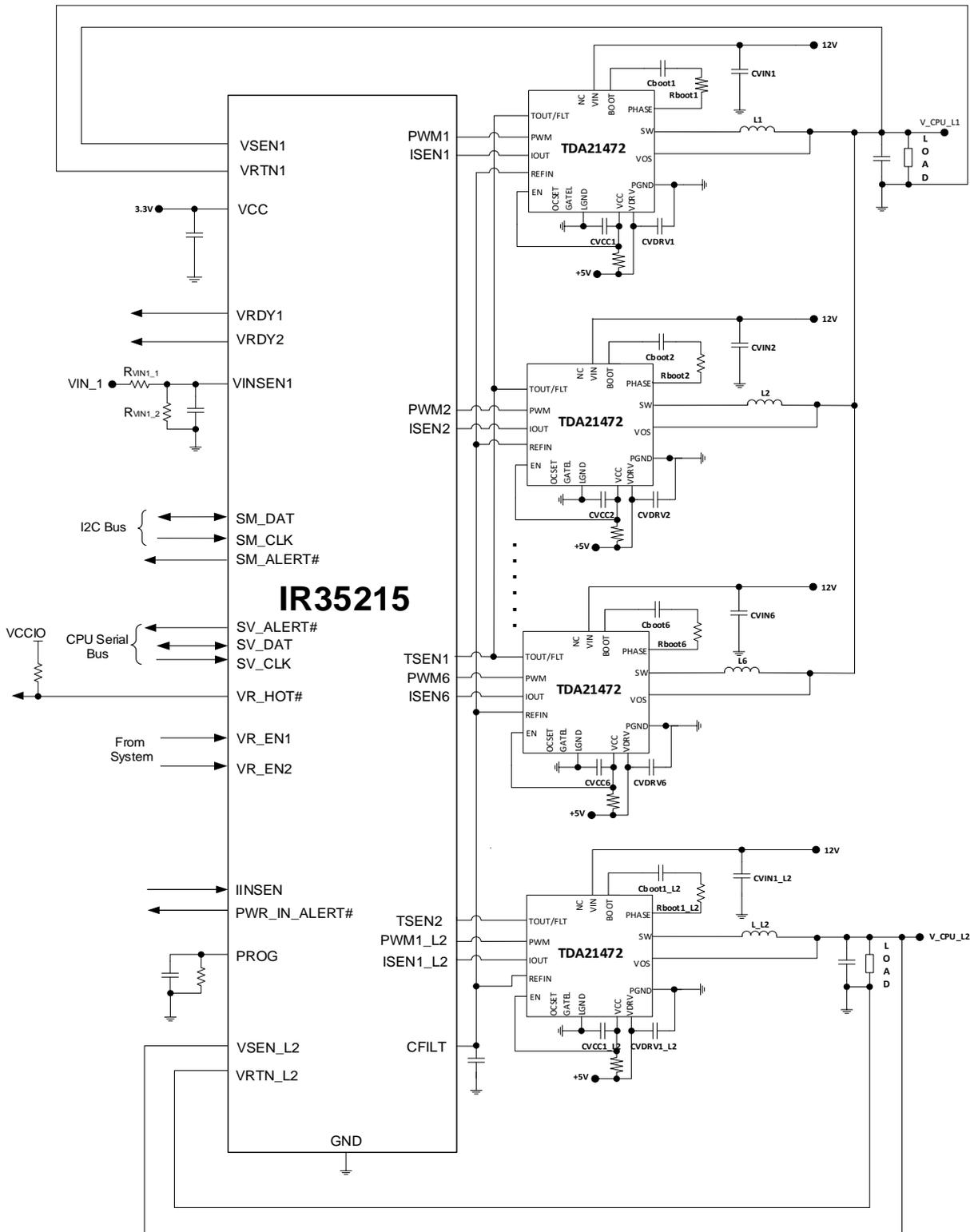
Figure 10 6+1 - Phase Voltage Regulator - Typical Application (simplified schematic)
