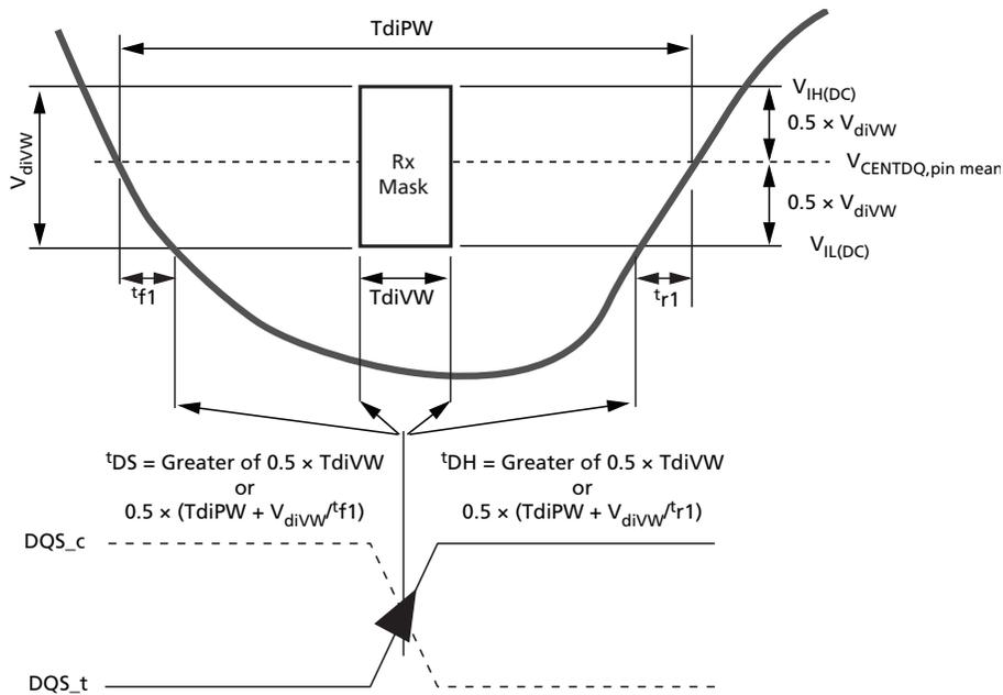
The following figure and table show an example of the worst case Rx mask required if the DQS and DQ pins do not have DRAM controller to DRAM write DQ training. The figure and table show that without DRAM write DQ training, the Rx mask would increase from 0.2UI to essentially 0.54UI. This would also be the minimum  $t_{DS}$  and  $t_{DH}$  required as well.
