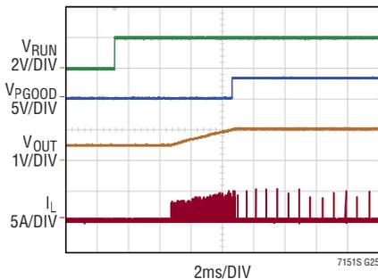
$V_{IN} = 12\text{V}$ ,  $C_{TRACK/SS} = 0.1\mu\text{F}$
