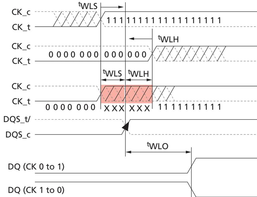
**DRAM Setting for Write Leveling and DRAM TERMINATION Function in that Mode**
