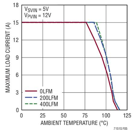
**Figure 5. Current Derating at 1MHz, 5V<sub>SVIN</sub>**
