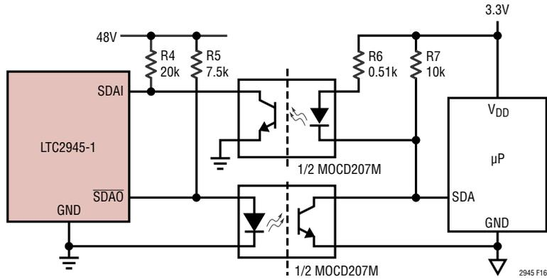
Figure 16. Opto-Isolation of a 1.5kHz I<sup>2</sup>C Interface Between LTC2945-1 and Microcontroller (SCL Omitted for Clarity)
