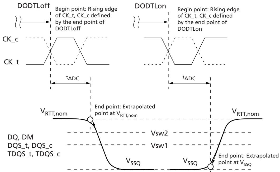
Figure 242:  $t_{ADC}$  Definition with Dynamic ODT Control
