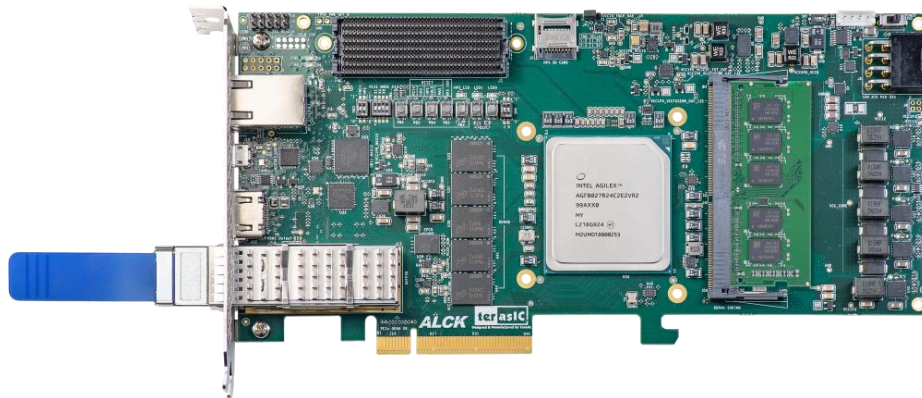
Figure 2-16 Setup QSFP28 loopback fixture
