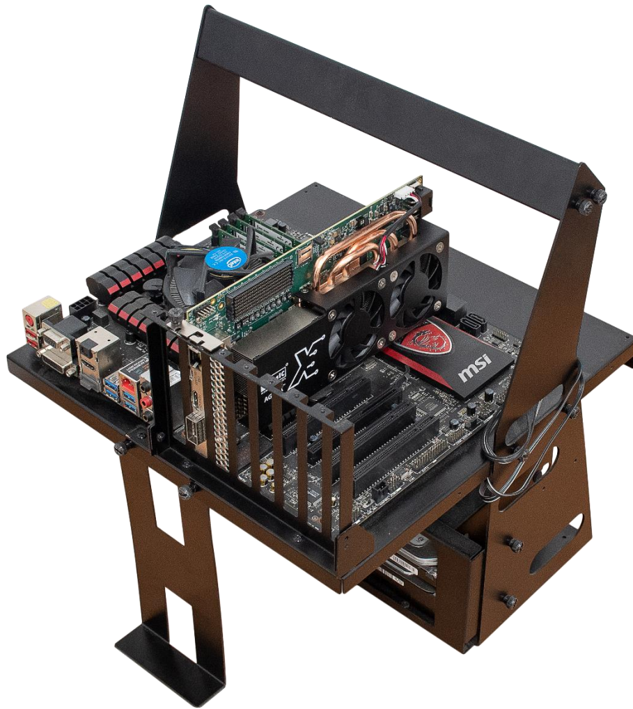
Figure 4-9 FPGA board installation on PC
