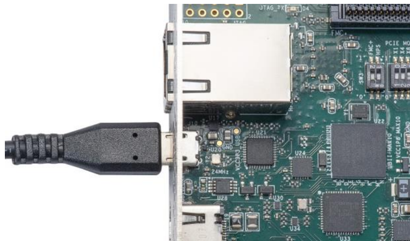
Figure 1-5 The Micro USB port
