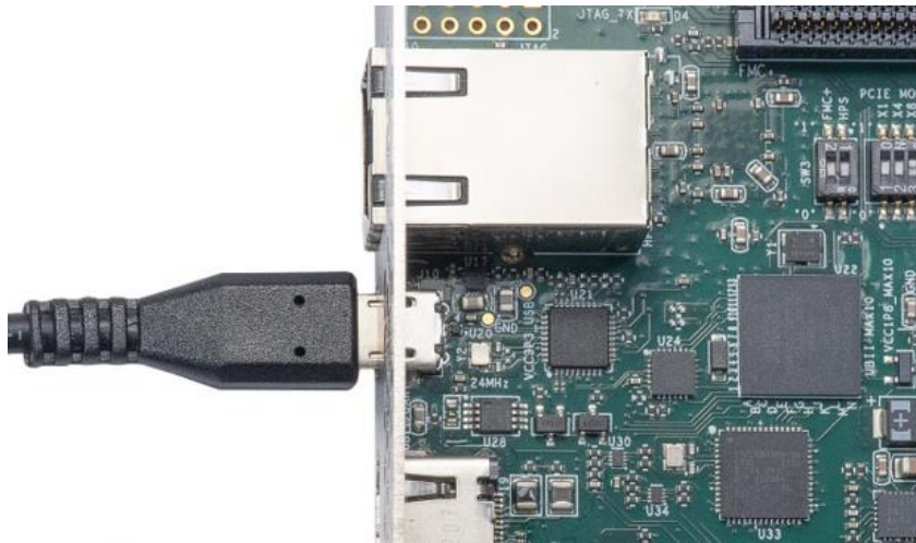
Figure 3-2 Connection setup for using dashboard system
