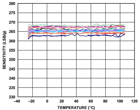
Figure 26. Y-Axis Sensitivity vs. Temperature—
