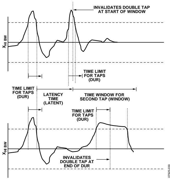
Figure 47. Tap Interrupt Function with Invalid Double Taps
