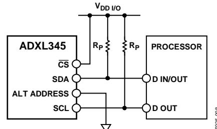
Figure 39. I<sup>2</sup>C Connection Diagram (Address 0x53)
