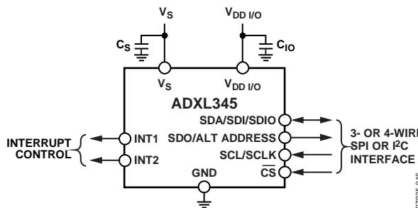
Figure 43. Application Diagram
