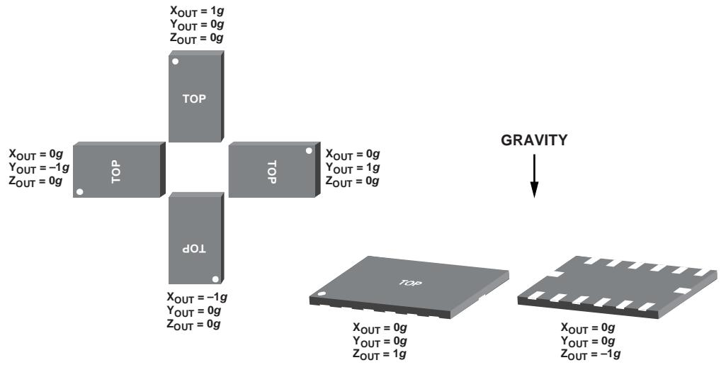
Figure 57. Output Response vs. Orientation to Gravity
