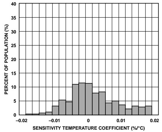
Figure 21. Z-Axis Sensitivity Temperature Coefficient,  $V_S = 2.5$  V
