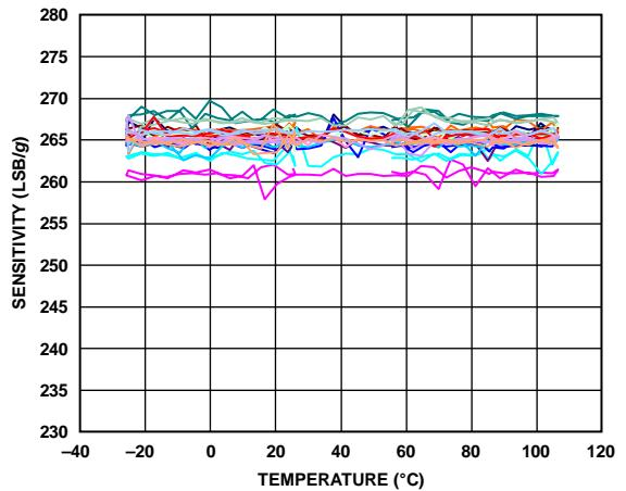
Figure 25. X-Axis Sensitivity vs. Temperature—
