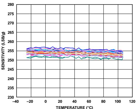
Figure 24. Z-Axis Sensitivity vs. Temperature—
