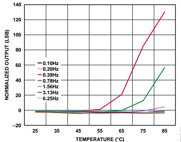
Figure 55. Typical Z-Axis Output vs. Temperature at Lower Data Rates,
