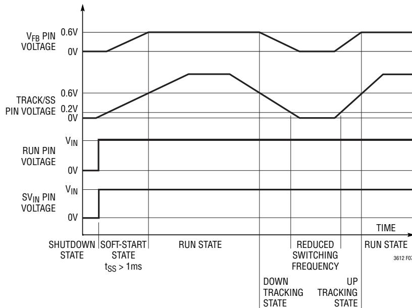
Figure 7. DDR Pin Not Tied to  $S_{VIN}$
