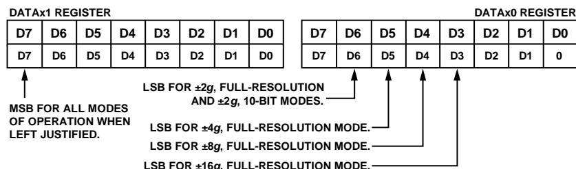
Figure 49. Data Formatting of Full-Resolution and  $\pm 2$  g, 10-Bit Modes of Operation When Output Data Is Left Justified
