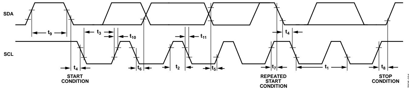
Figure 41. I<sup>2</sup>C Timing Diagram
