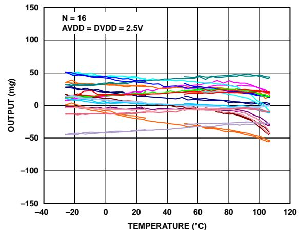
Figure 13. X-Axis Zero g Offset vs. Temperature—
