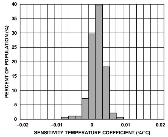
Figure 20. Y-Axis Sensitivity Temperature Coefficient,  $V_S = 2.5$  V
