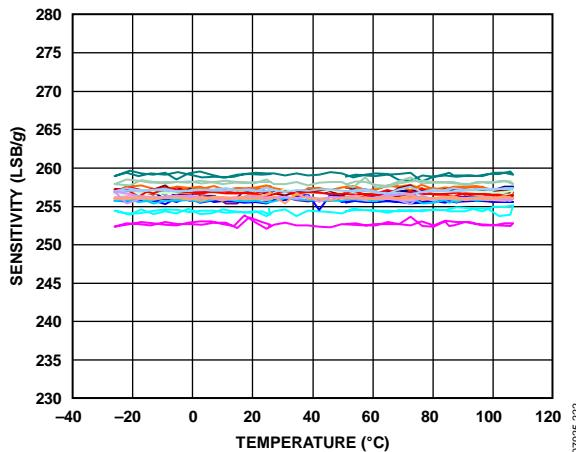
Figure 22. X-Axis Sensitivity vs. Temperature—
