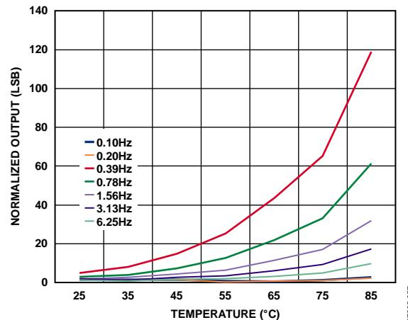
Figure 54. Typical Y-Axis Output vs. Temperature at Lower Data Rates,
