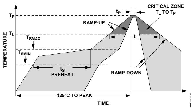
Figure 59. Recommended Soldering Profile
