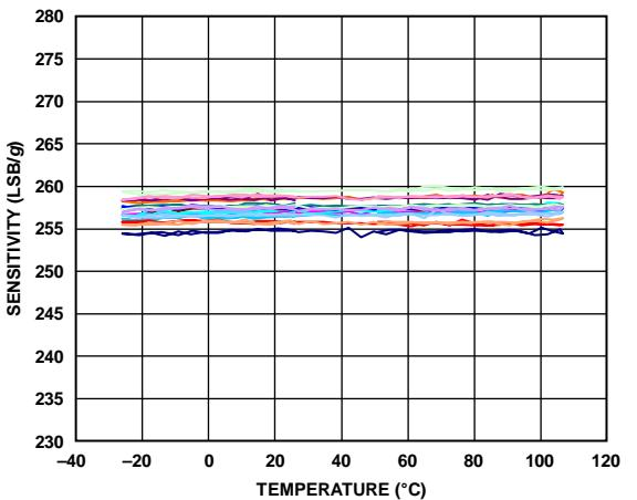
Figure 23. Y-Axis Sensitivity vs. Temperature—
