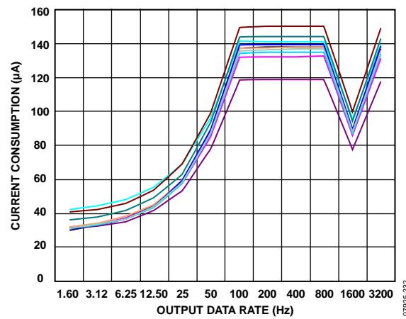
Figure 32. Current Consumption vs. Output Data Rate at 25°C—10 Parts,  $V_s = 2.5\text{ V}$
