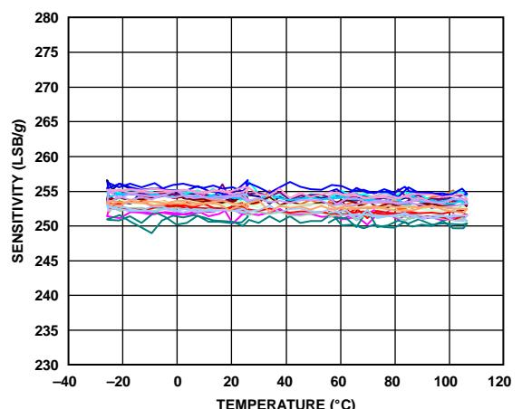
Figure 27. Z-Axis Sensitivity vs. Temperature—
