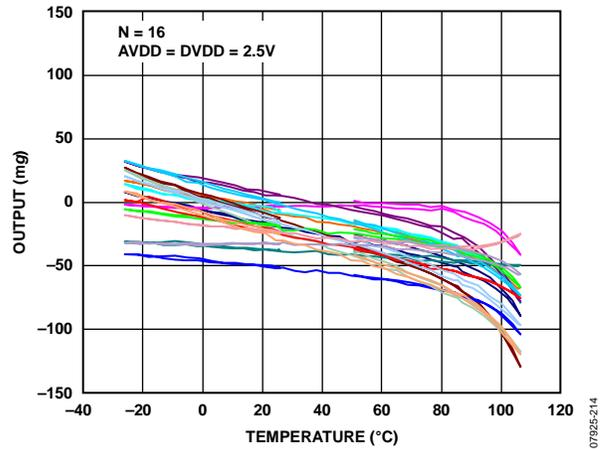
Figure 14. Y-Axis Zero g Offset vs. Temperature—
