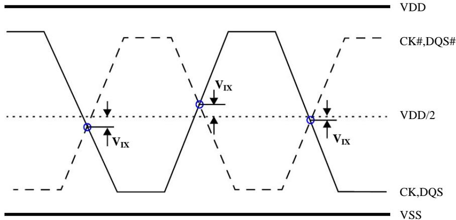
Figure 4.4.  $V_{ix}$  Definition
