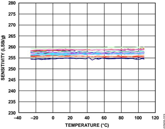
Figure 23. Y-Axis Sensitivity vs. Temperature—
