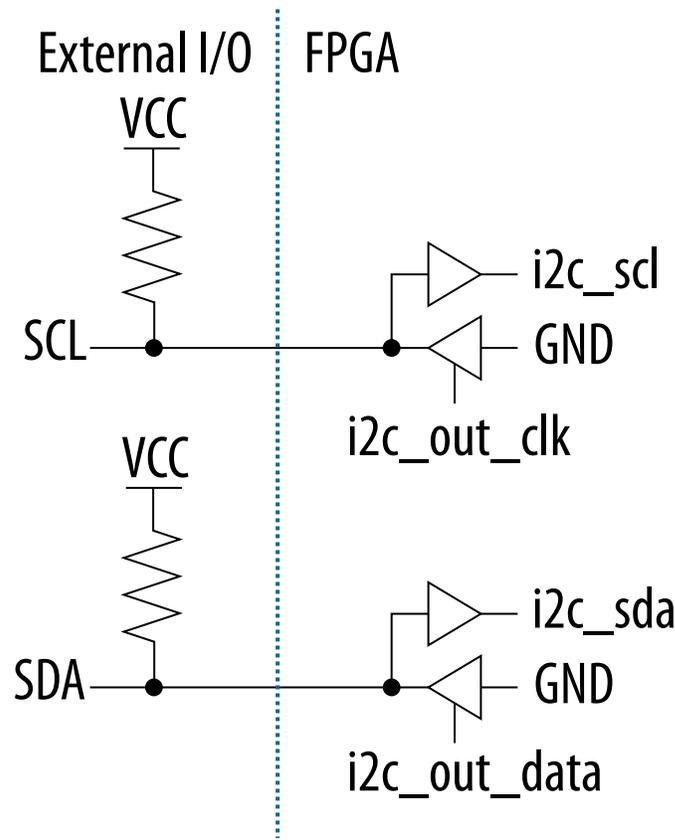
The figure above shows the typical connection on the I<sup>2</sup>C interface in FPGA fabric with `alt_iobuff`.
