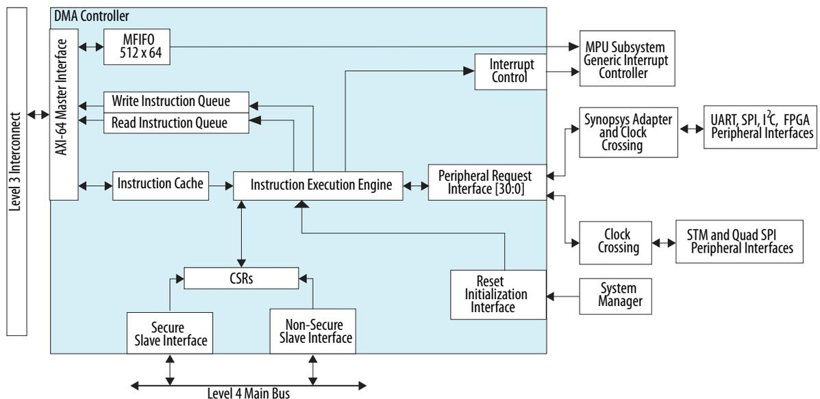
The `14_main_clk` clock drives the DMA controller, controller logic, and all the interfaces. The DMA controller accesses the level 3 (L3) main switch with its 64-bit AXI master interface.
