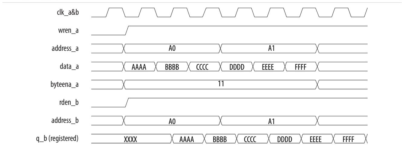
**Figure 2-4: Mixed-Port Read-During-Write: Old Data Mode**
