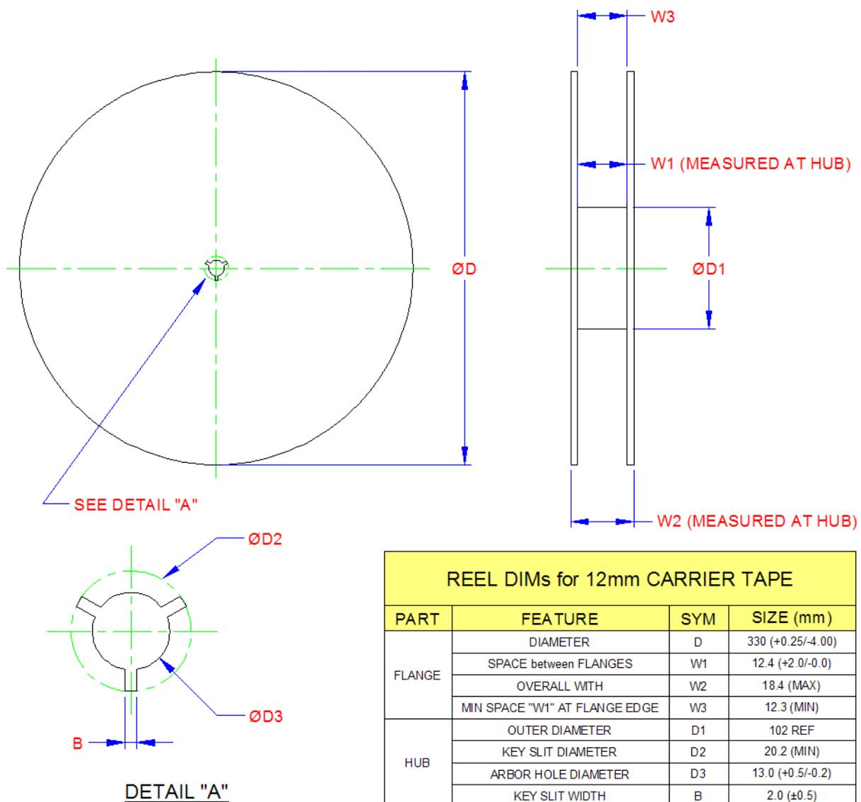
**Figure 8.2 Reel Dimensions for 12mm Carrier Tape**
