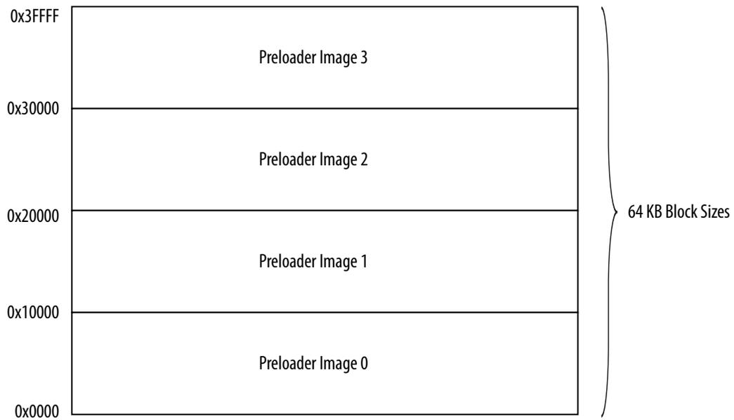
Figure A-7: NAND Flash Image Layout for 128 KB Memory Blocks
