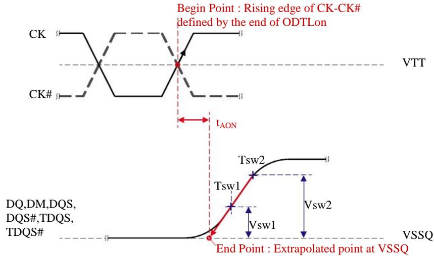
Figure 5.9.2.2 Definition of  $t_{AONPD}$
