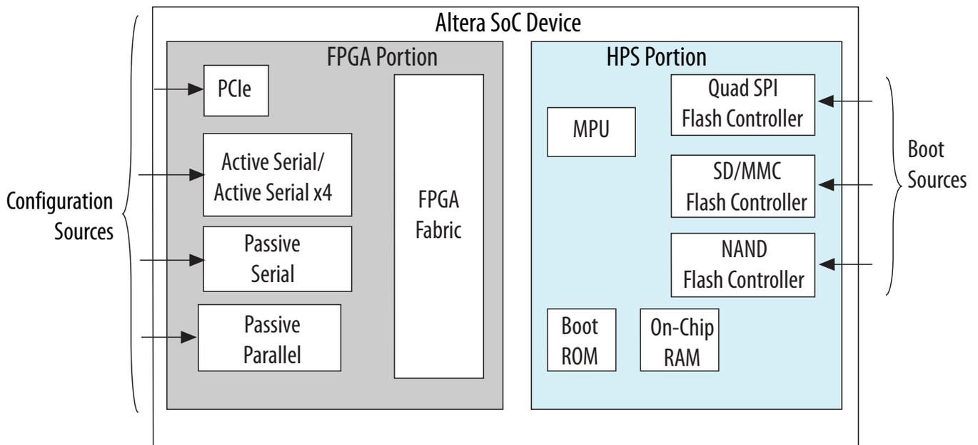
In the figure below, the FPGA is configured first through one of its non-HPS configuration sources and then the HPS executes the second-stage boot loader from the FPGA. The HPS boot ROM waits for the FPGA fabric to be powered on and in user mode before executing. The HPS boot ROM code executes the second-stage boot loader from the FPGA fabric over the HPS-to-FPGA bridge.
