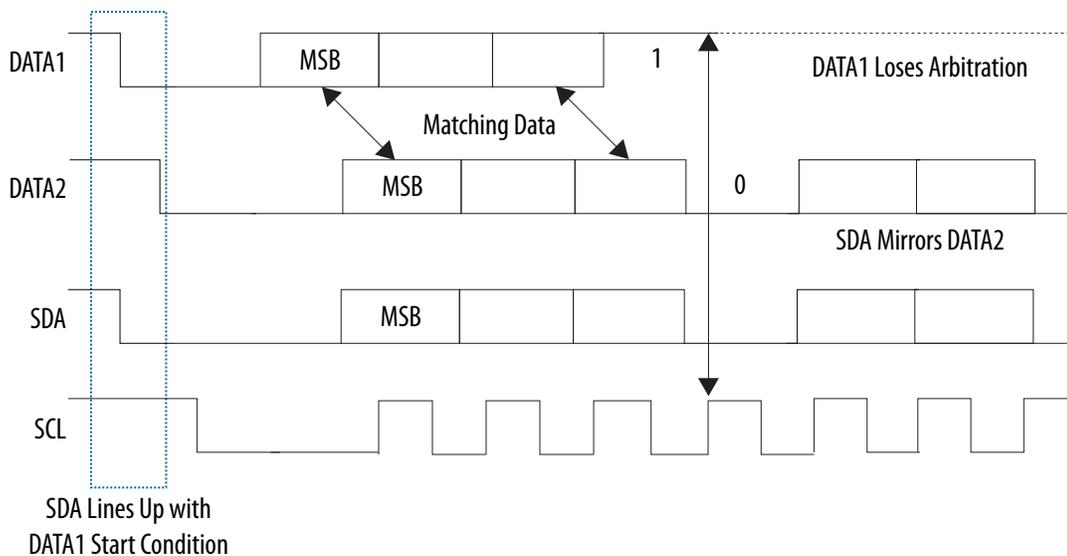
The bus control is determined by address or master Data code and data sent by competing masters, so there is no central master nor any order of priority on the bus. †
