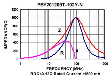
Test Instruments : Agilent E4991A Impedance / Material Analyzer
