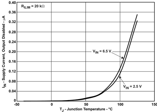
Figure 18.  $I_{IN}$  – Supply Current, Output Disabled –  $\mu A$
