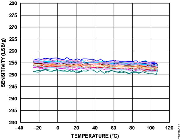
Figure 24. Z-Axis Sensitivity vs. Temperature—
