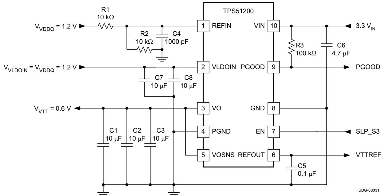
**Figure 28. 3.3- $V_{IN}$ , LP DDR3 Configuration**
