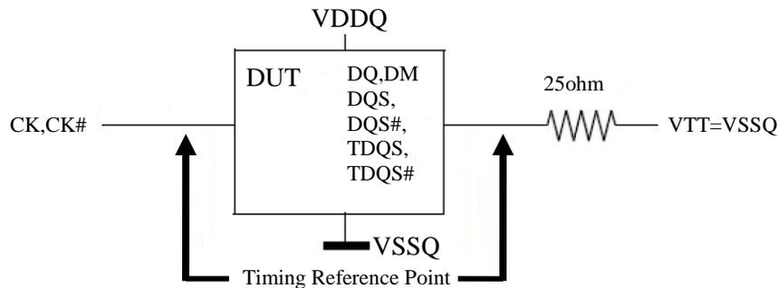
Figure 5.9.1 ODT Timing Reference Load
