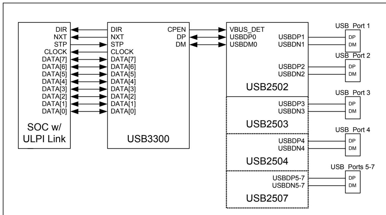
**Figure 7.4 Expanding Downstream Ports for USB3300 Host Applications**
