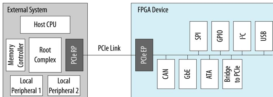
The Cyclone V PCIe hard IP operates independently from the core logic. This independent operation allows the PCIe link to wake up and complete link training in less than 100 ms while the Cyclone V device completes loading the programming file for the rest of the device.
