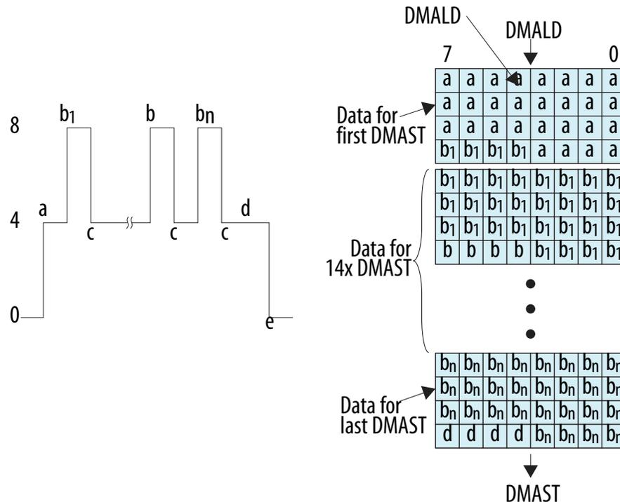
**Note:** The `DMALD` shown as `a` does not increase the MFIFO buffer usage because it loads four bytes into an MFIFO buffer entry that the DMAC has already allocated to this channel.
