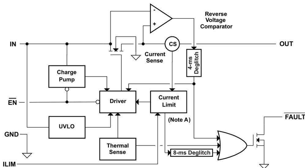
Note A: TPS255x parts enter constant current mode during current limit condition; TPS255x-1 parts latch off
