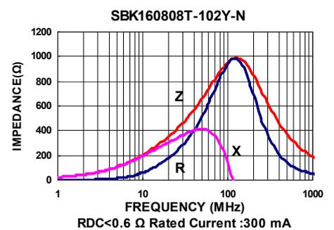
Test Instruments : Agilent E4991A Impedance / Material Analyzer
