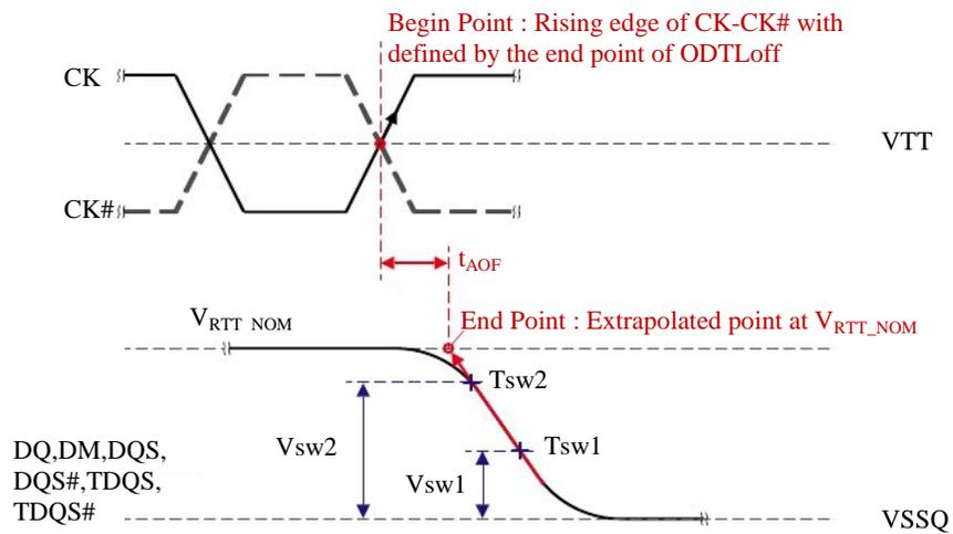
Figure 5.9.2.4 Definition of  $t_{AOFPD}$
