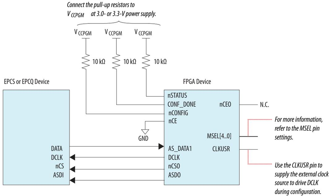
Figure 7-6: Single Device AS x4 Mode Configuration
