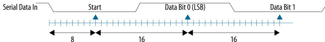
The baud rate of the UART controller is controlled by the serial clock and the Divisor Latch Register (DLH and DLL).†
