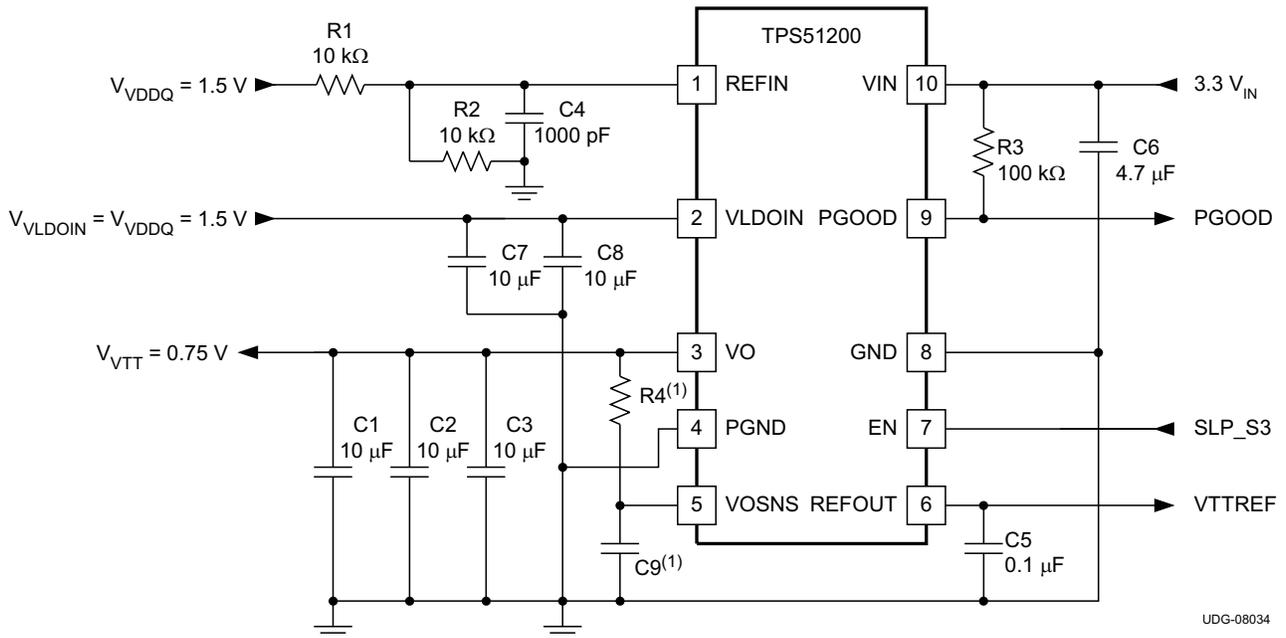
**Figure 31. 3.3- $V_{IN}$ , DDR3 Configuration with LFP**
