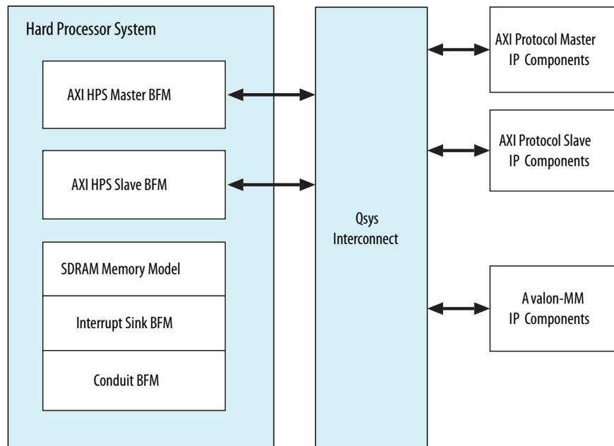
The HPS BFM uses standard function calls from the Altera BFM application programming interface (API), as detailed in the remainder of this chapter.
