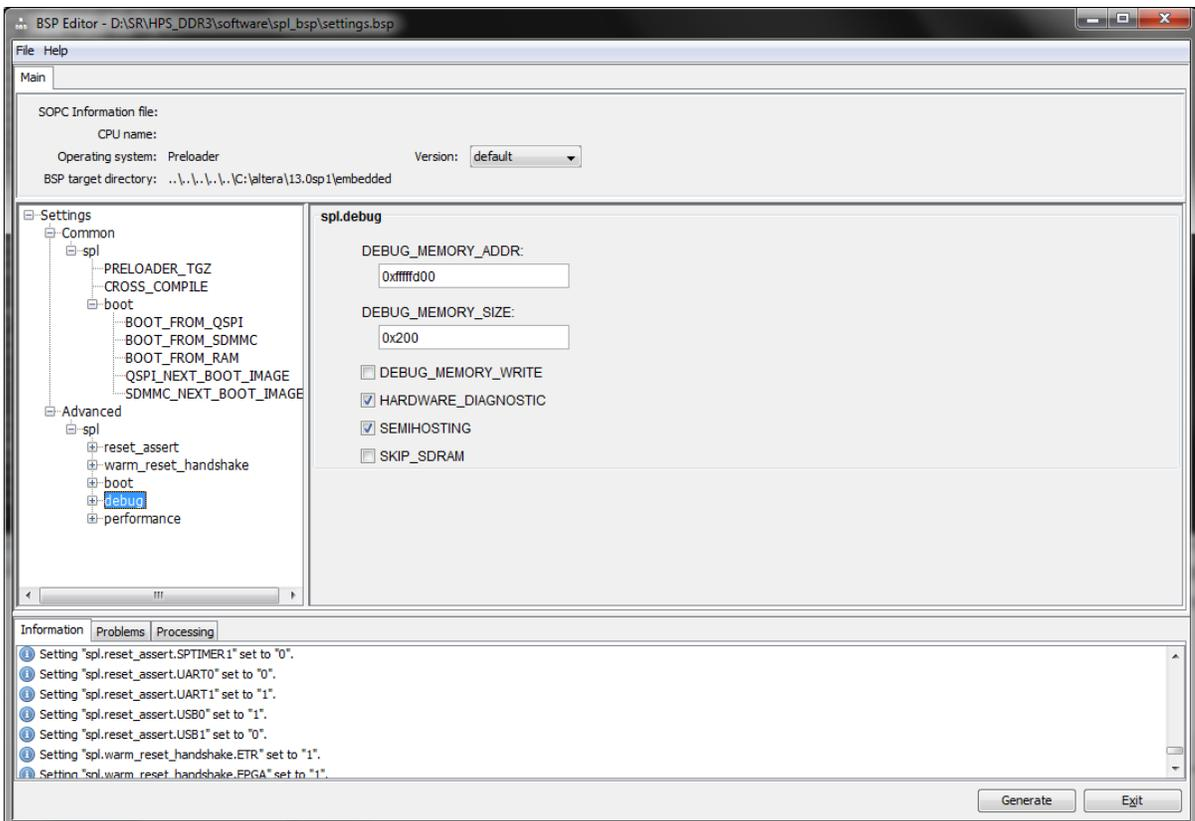
2. The simple memory test assumes SDRAM with a memory size of 1 GB. If your board contains a different SDRAM memory size, open the file **<design folder>\spl\_bsp\uboot-socfpga\include\configs\**
