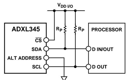
Figure 39. I<sup>2</sup>C Connection Diagram (Address 0x53)
