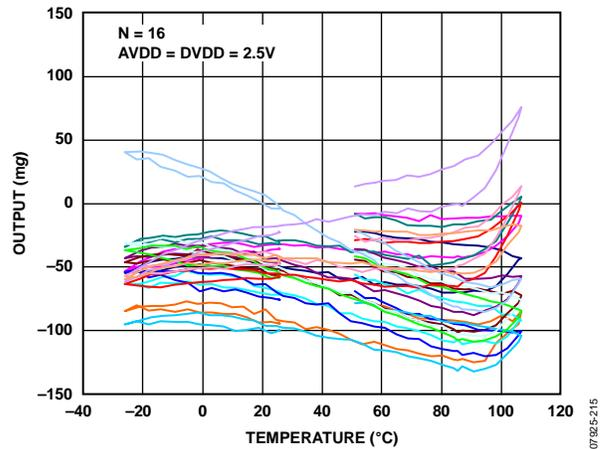
Figure 15. Z-Axis Zero g Offset vs. Temperature—
