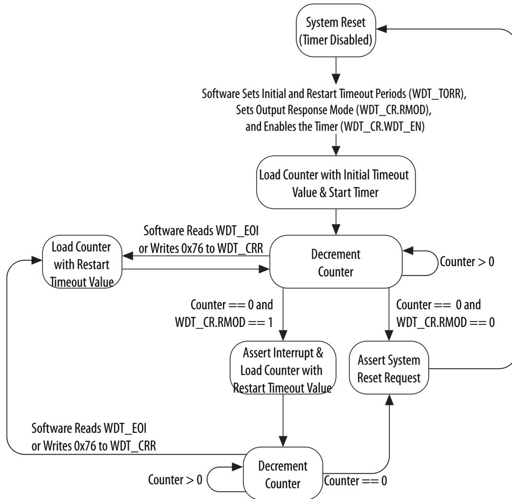
If the counter reaches zero, the state changes based on the value of the output response mode setting defined in the `rmod` bit of the `wdt_cr` register. If the `rmod` bit of the `wdt_cr` register is 0, the output response mode is to generate a system reset request. In this case, the state changes to Assert System Reset Request. In response, the reset manager resets and disables the watchdog timer, and gives software the opportunity to reinitialize the timer.
