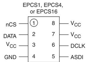
Figure 14–21 shows the Altera serial configuration device 16-pin SOIC package and its pin-out diagram.
