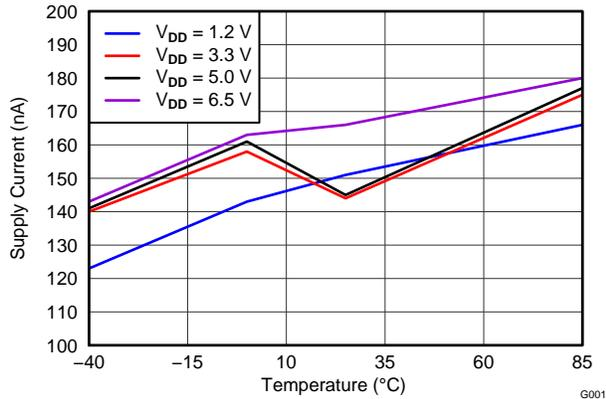
Figure 4. SUPPLY CURRENT vs INPUT VOLTAGE AND TEMPERATURE
