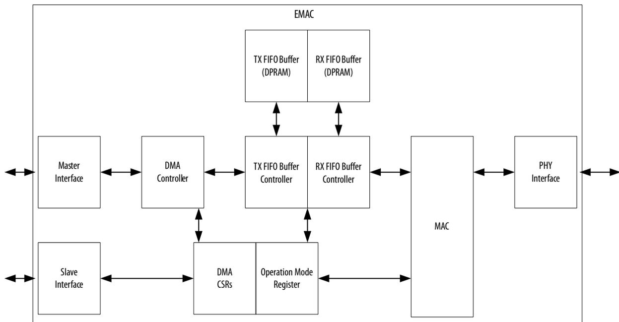
There are two host interfaces to the Ethernet MAC. The management host interface, a 32-bit slave interface, provides access to the CSR set regardless of whether or not the EMACs are used directly through the FPGA fabric. The data interface is a 32-bit master interface, and it controls data transfer between the direct memory access (DMA) controller channels and the rest of the HPS system through the system interconnect.
