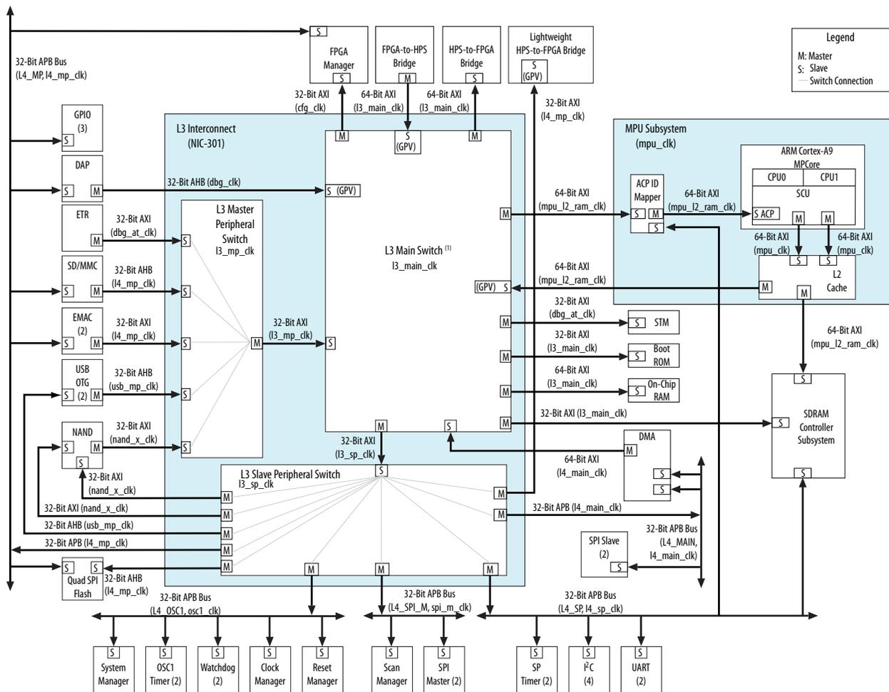
**Note:** System interconnect slaves are available for connection from peripheral masters. System interconnect masters connect to peripheral slaves. This terminology is the reverse of conventional terminology used in Qsys.
