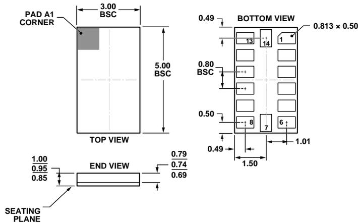
Figure 60. 14-Terminal Land Grid Array [LGA]
