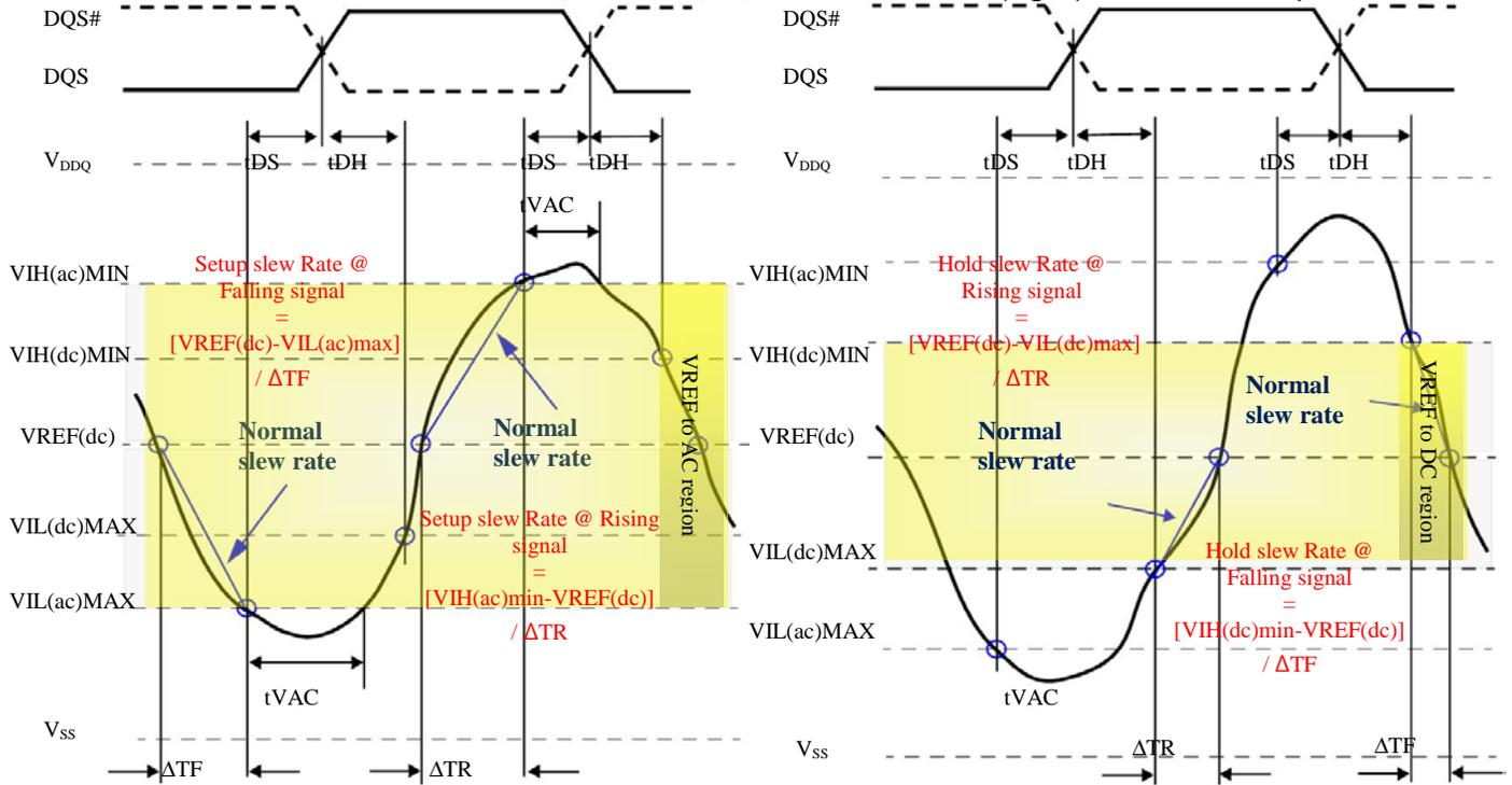
9.6.5.2 Tangent line for setup time tDS(left) and hold time tDH(right) - DQ with respect to strobe
