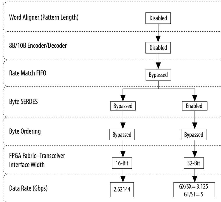
**Figure 5-11: Configuration Options for Low Latency Custom Double-Width Mode (20-bit PMA–PCS Interface Width)**
