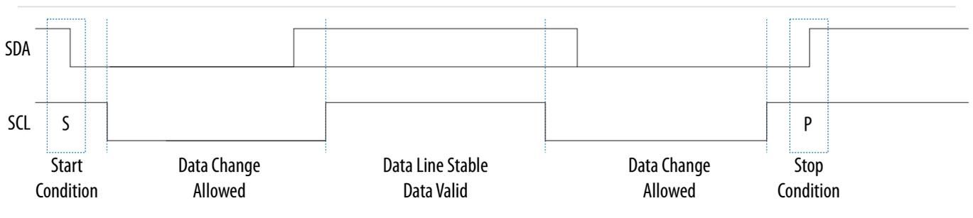
The signal transitions for the START or STOP condition, as shown in the figure, reflect those observed at the output signals of the master driving the I<sup>2</sup>C bus. Care should be taken when observing the SDA or SCL signals at the input signals of the slave(s), because unequal line delays may result in an incorrect SDA or SCL timing relationship. †
