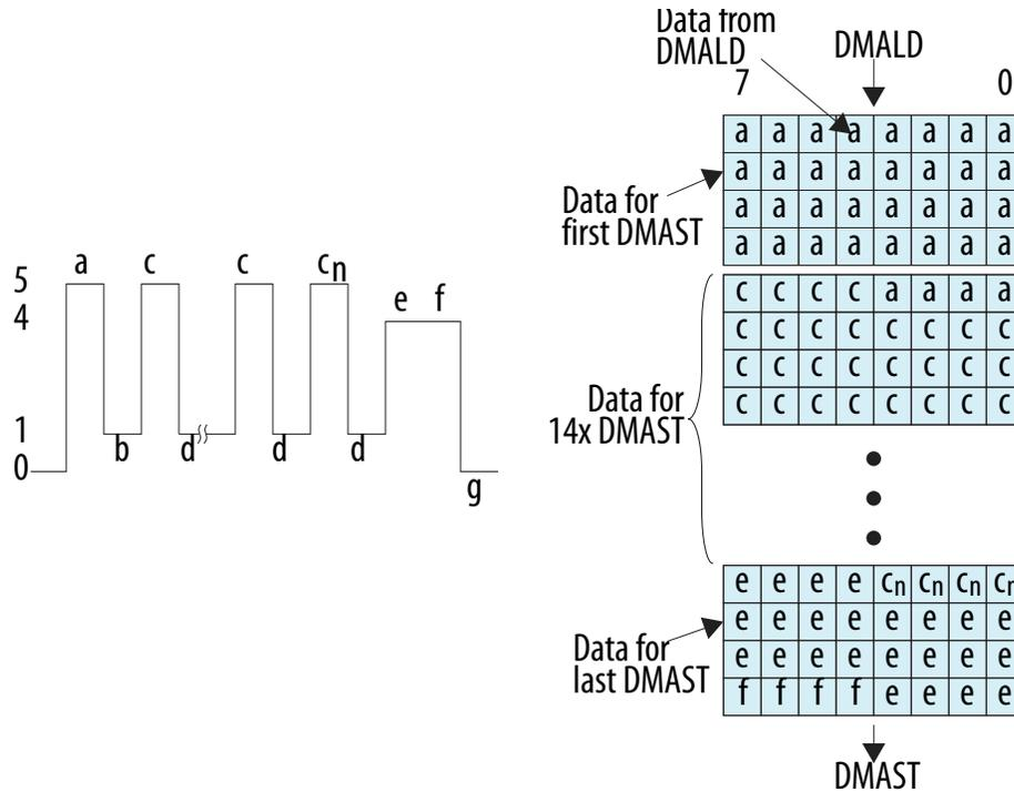
**Note:** The DMALD shown as **f** does not increase the MFIFO buffer usage because it loads four bytes into an MFIFO buffer entry that the DMAC has already allocated to this channel.
