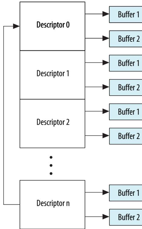
Figure 17-5: Descriptor Chain Structure
