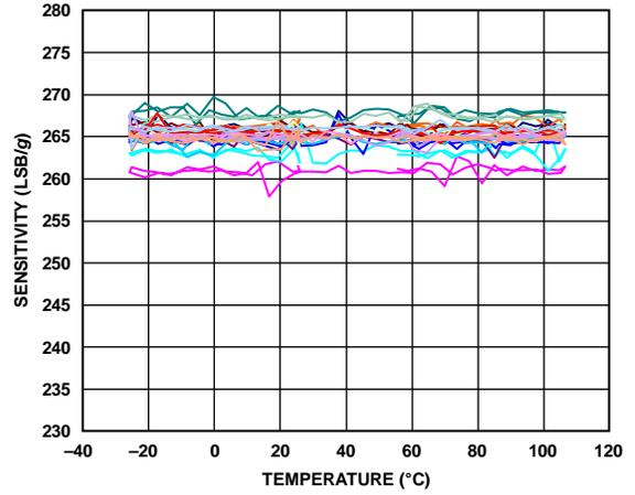
Figure 25. X-Axis Sensitivity vs. Temperature—
