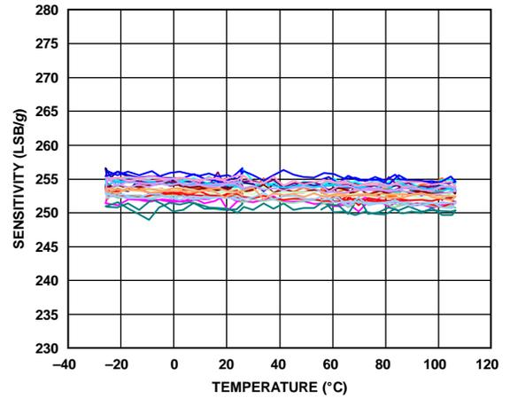
Figure 27. Z-Axis Sensitivity vs. Temperature—
