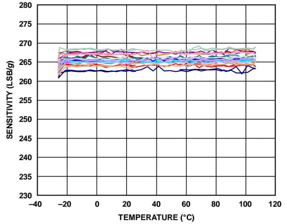
Figure 26. Y-Axis Sensitivity vs. Temperature—
