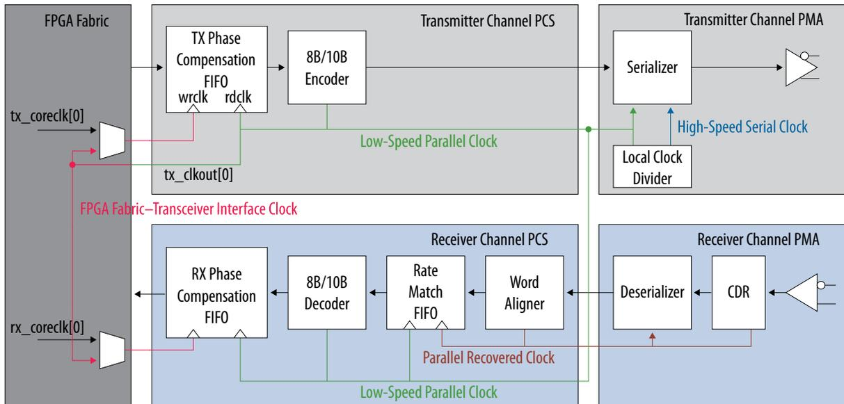
Figure 4-15: Transceiver Datapath in GbE-3.125 Gbps Configuration
