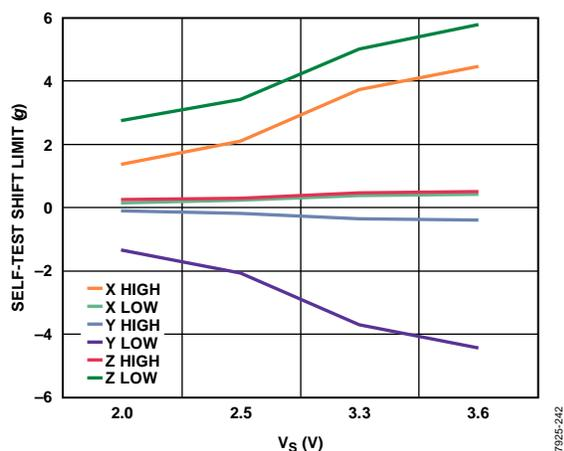
Figure 42. Self-Test Output Change Limits vs. Supply Voltage
