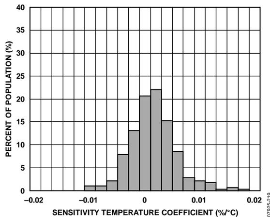
Figure 19. X-Axis Sensitivity Temperature Coefficient,  $V_S = 2.5 V$
