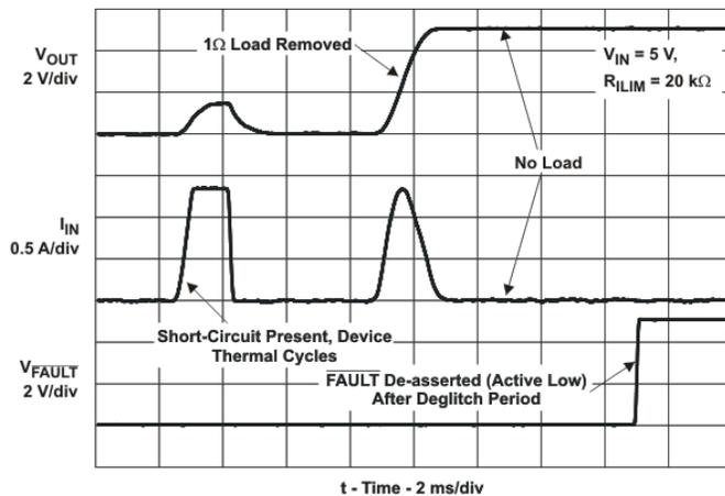
Figure 14. 1Ω to No Load Transient Response
