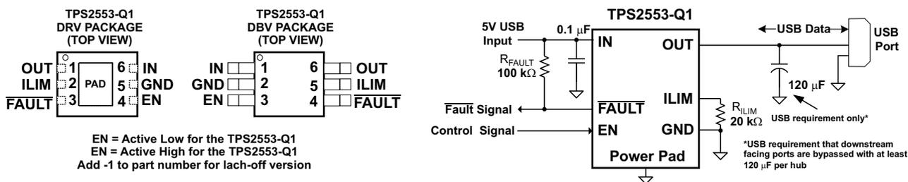
Figure 1. Typical Application as USB Power Switch
