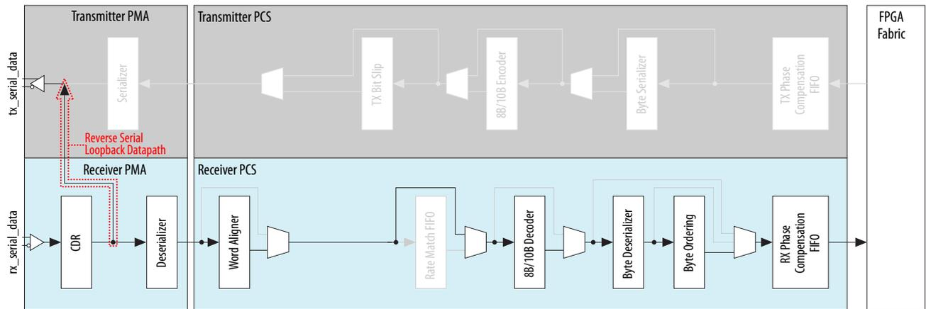
Note: Grayed-out blocks are not active when the reverse serial loopback is enabled.
