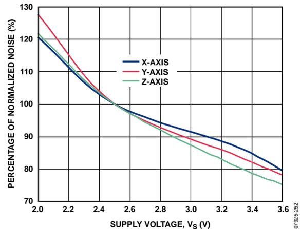
Figure 52. Normalized Noise vs. Supply Voltage,  $V_s$
