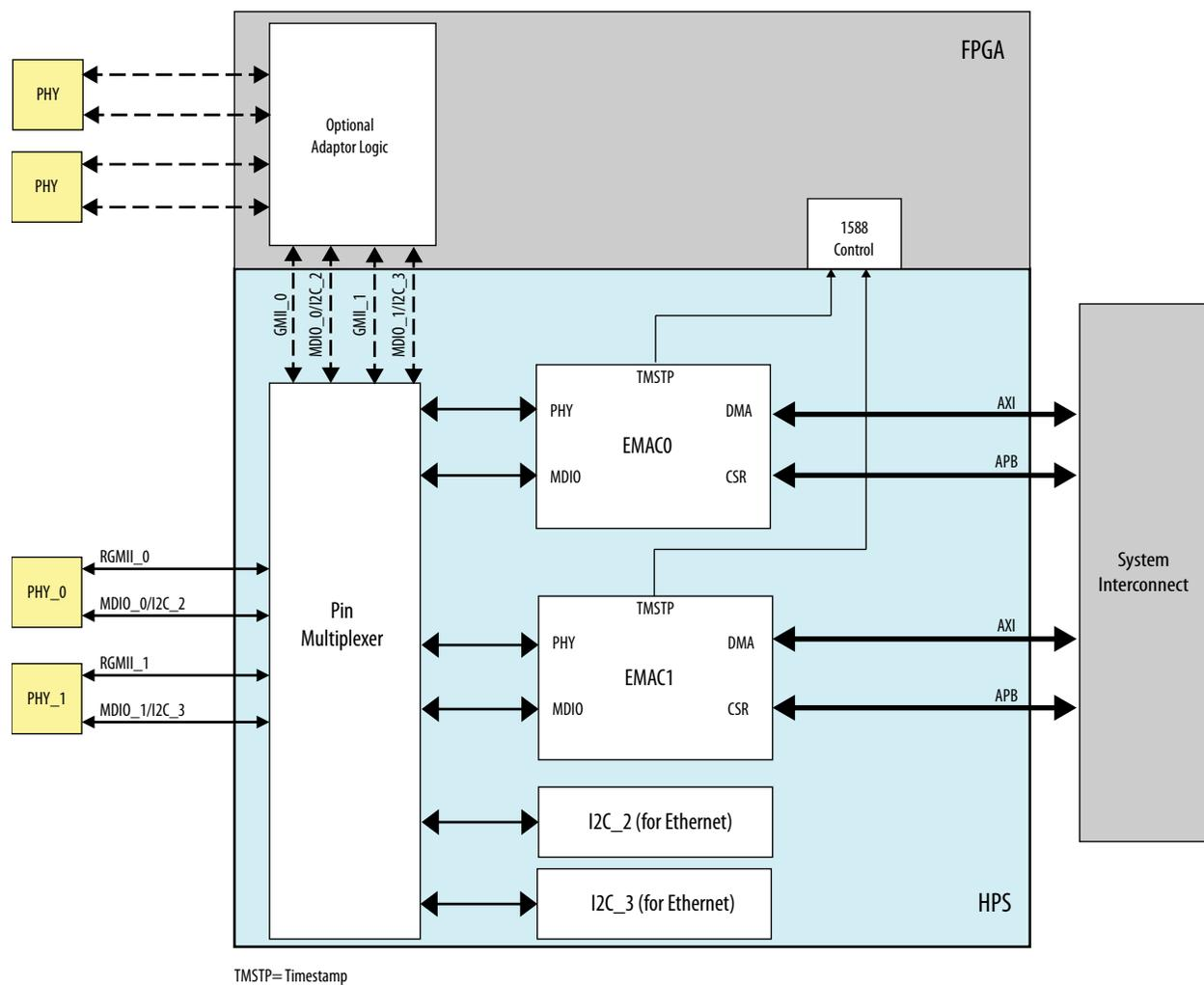
The EMACs are integrated into the HPS portion of the system on a chip (SoC) device. They communicate with the I/O pins.
