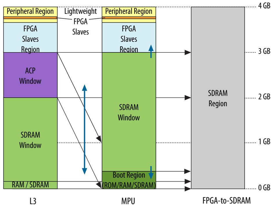
The window regions provide access to other address spaces. The thin black arrows indicate which address space is accessed by a window region (arrows point to accessed address space). For example, accesses to the ACP window in the L3 address space map to a 1 GB region of the MPU address space.
