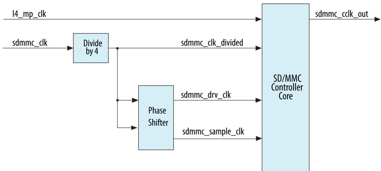
The `sdmmc_clk` clock from the clock manager is divided by four and becomes the `sdmmc_clk_divided` clock before passing to the phase shifters and the SD/MMC controller CIU. The phase shifters are used to generate the `sdmmc_drv_clk` and `sdmmc_sample_clk` clocks. These phase shifters provide up to eight phases shift which include 0, 45, 90, 135, 180, 225, 270, and 315 degrees. The `sdmmc_sample_clk` clock can be driven by the output from the phase shifter.
