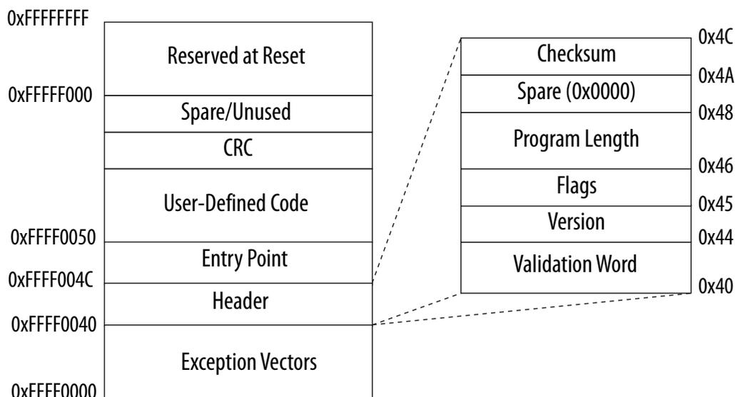
**Exception vectors**—Exception vectors are located at the start of the on-chip RAM. Typically, the second-stage boot loader remaps the lowest region of the memory map to the on-chip RAM (from the boot ROM) to create easier access to the exception vectors.
