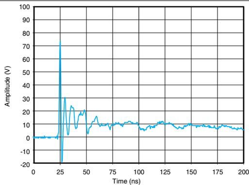
Figure 5. IEC Clamping Waveforms (8 kV Contact)
