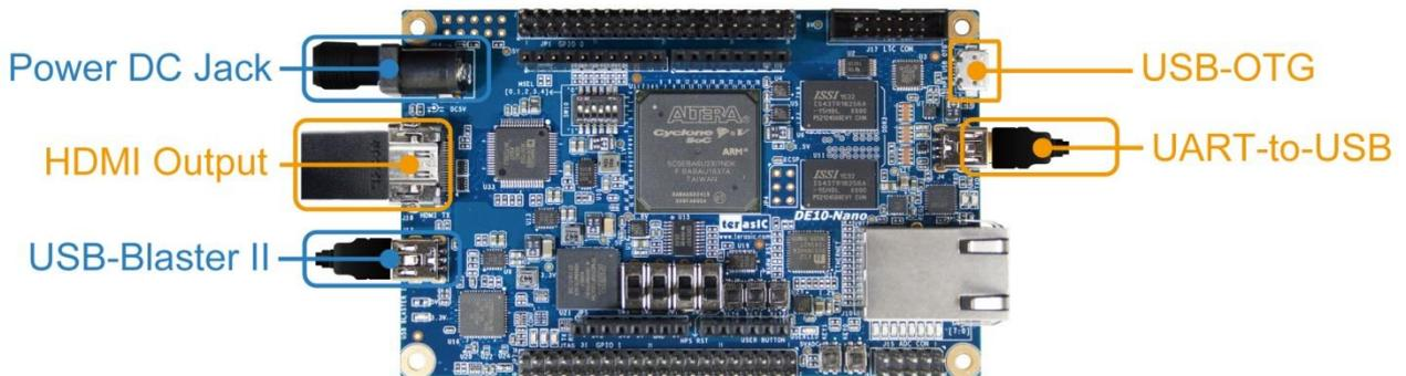
Figure 2-3 USB, HDMI Output and Power Cables
