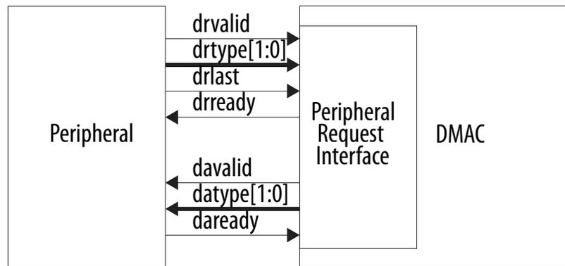
The peripheral indicates the following on the request bus:
