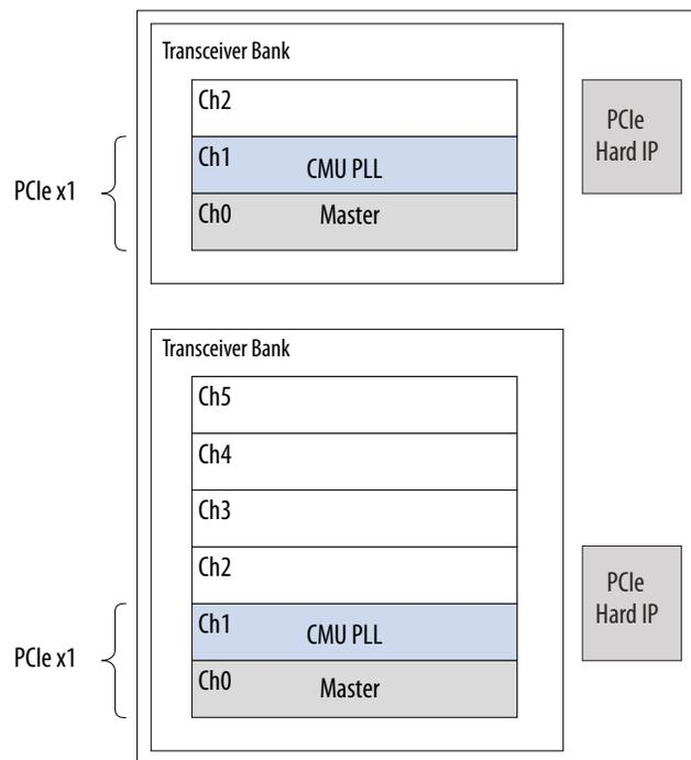
**Figure 4-9: 6 Transceiver Channels and 1 PCIe HIP Blocks with PCIe x2 and x4 Channel Placement**
