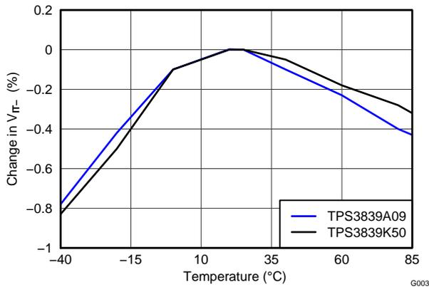
Figure 6. PERCENTAGE CHANGE IN THRESHOLD VOLTAGE vs TEMPERATURE
