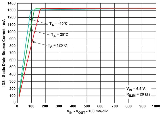
Figure 22. Switch Current Vs. Drain-Source Voltage Across Switch
