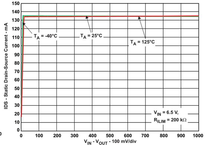
Figure 23. Switch Current Vs. Drain-Source Voltage Across Switch
