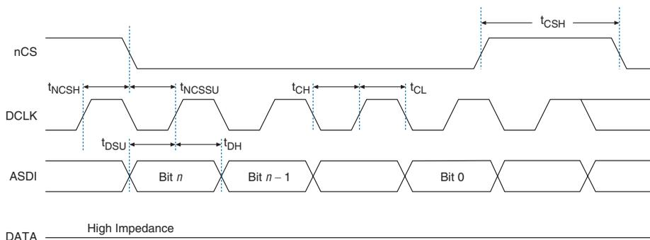
Table 14–23 defines the serial configuration device timing parameters for write operation.
