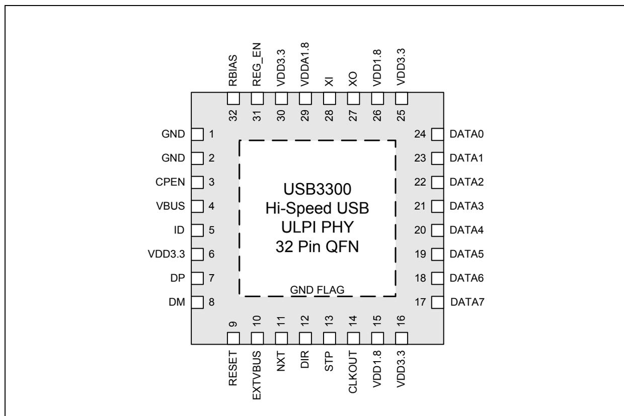
Figure 3.1 USB3300 Pin Diagram - Top View
