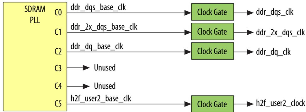
The SDRAM PLL output clocks can be phase shifted in real time in increments of 1/8 the VCO frequency. Maximum number of phase shift increments is 4096.
