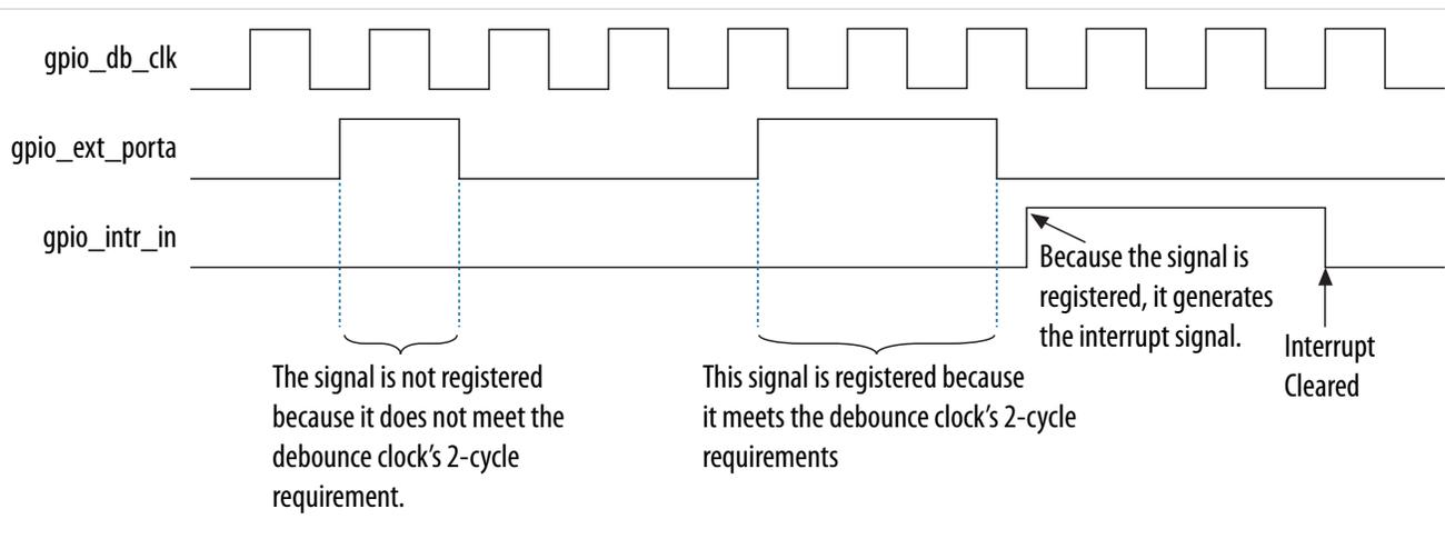
**Note:** Enabling the debounce circuitry increases interrupt latency by two clock cycles of the debounce clock.
