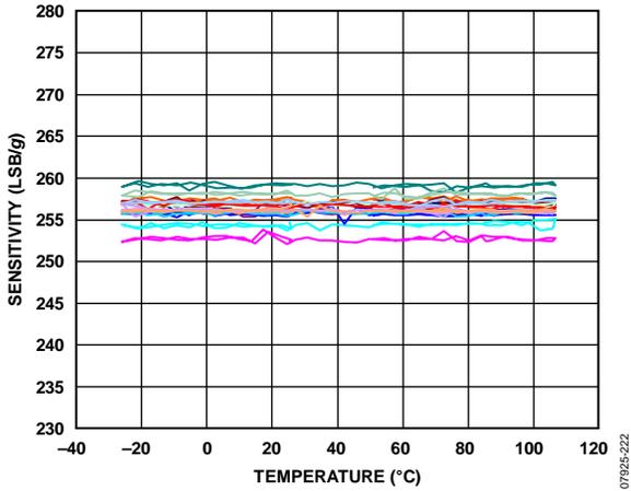
Figure 22. X-Axis Sensitivity vs. Temperature—
