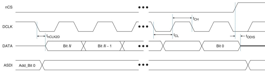
Table 14–24 defines the serial configuration device timing parameters for read operation.
