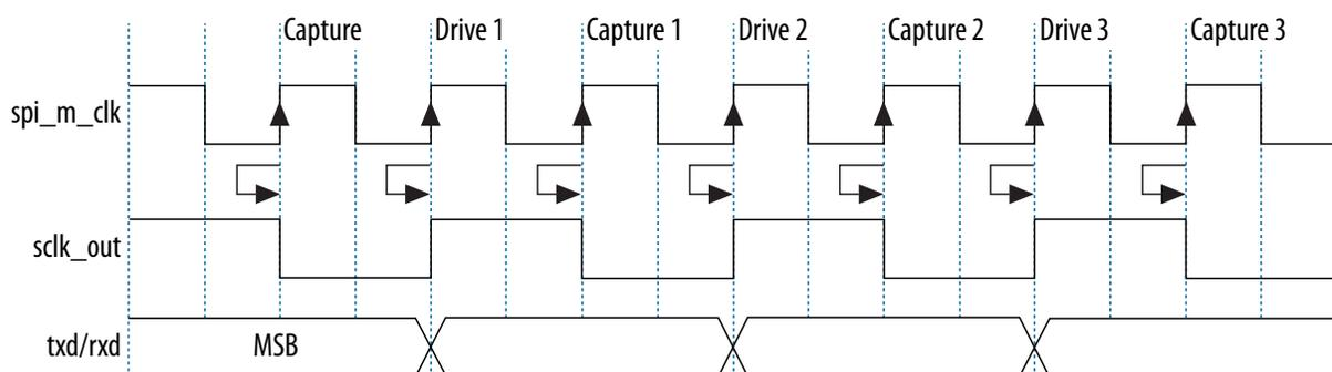
The frequency of `sclk_out` can be derived from the equation below, where `<SPI clock>` is `spi_m_clk` for the master SPI modules and `l4_main_clk` for the slave SPI modules. †
