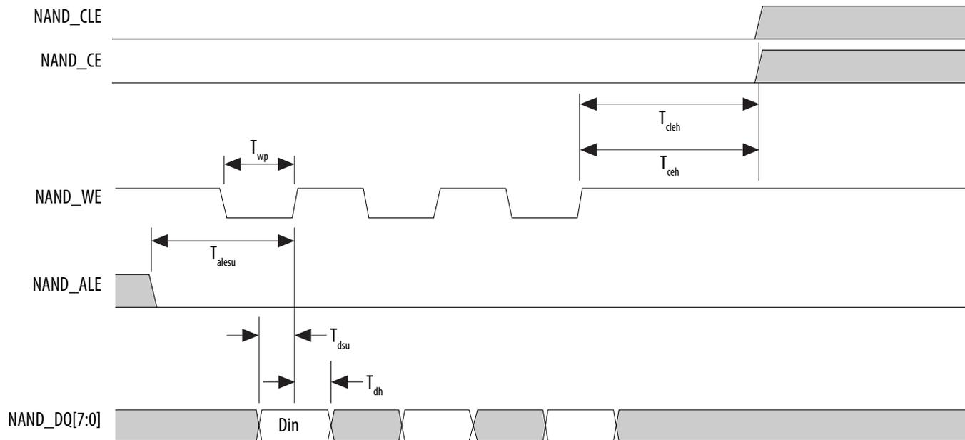
Figure 17: NAND Data Read Timing Diagram
