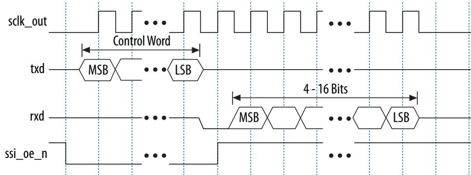
Figure 19-12: Single SPI Slave Microwire Serial Transfer (MDD=1)
