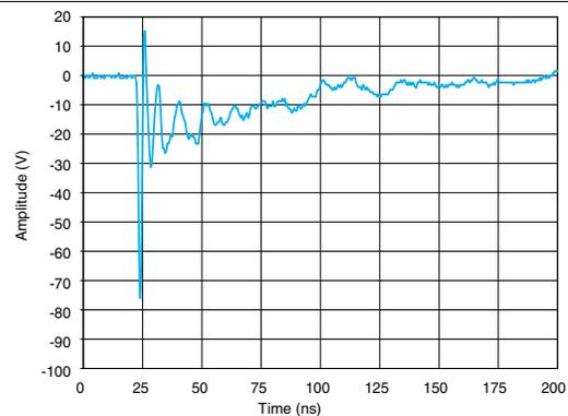
Figure 6. IEC Clamping Waveforms (-8 kV Contact)
