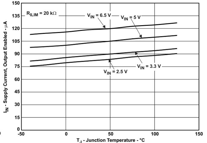
Figure 19.  $I_{IN}$  – Supply Current, Output Enabled –  $\mu A$
