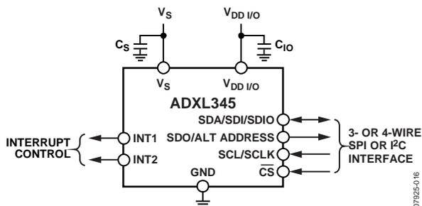
Figure 43. Application Diagram
