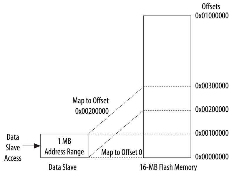
To remap the data slave to access other 1 MB regions of the flash device, enable address remapping in the enable ARM® AMBA® advanced high speed bus (AHB) address remapping field (`enahbremap`) of the `cfg` register. All incoming data slave accesses remap to the offset specified in the remap address register (`remapaddr`).
