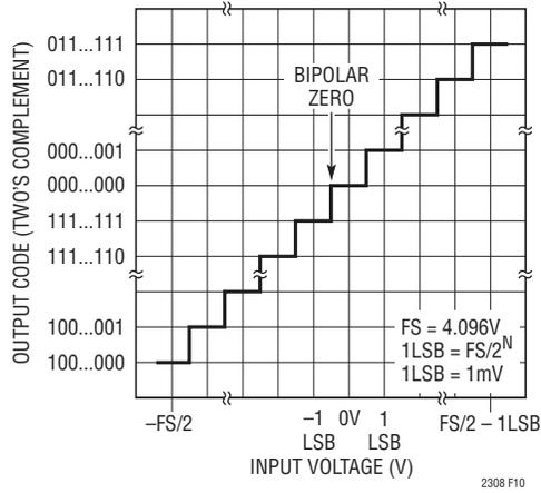
Figure 10. LTC2308 Bipolar Transfer Characteristics (2's Complement)
