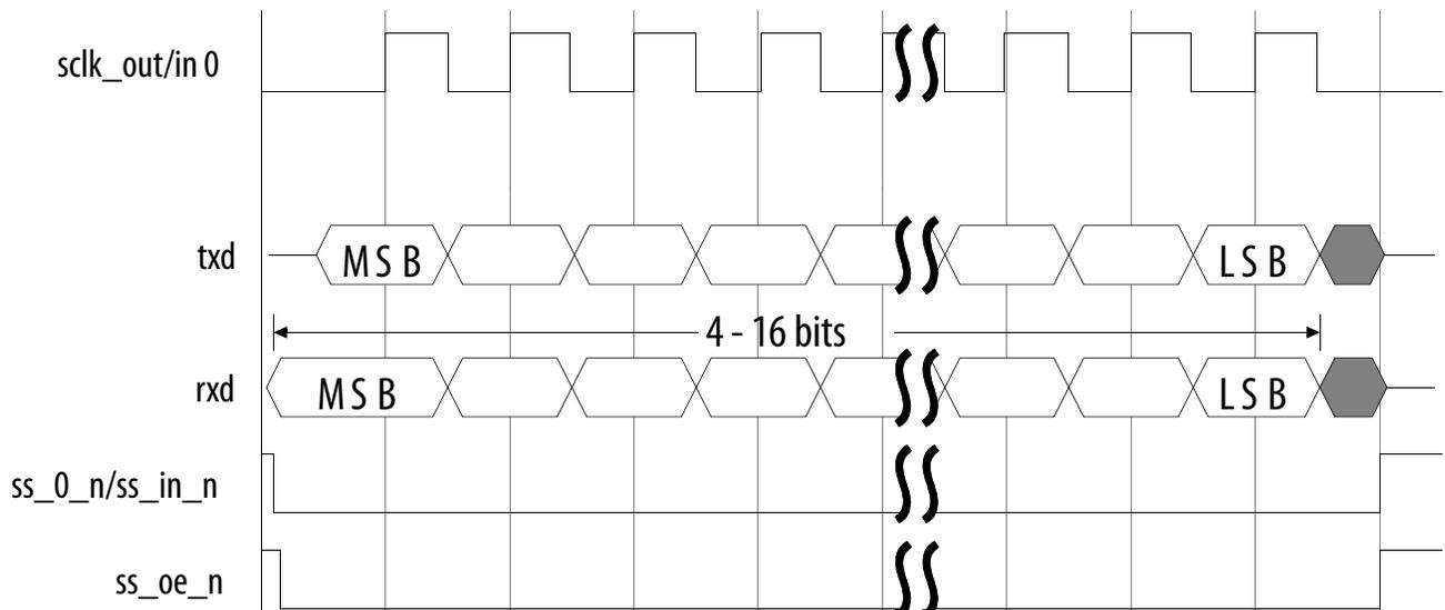
There are four possible transfer modes on the SPI controller for performing SPI serial transactions; refer to “Transfer Modes”. For *transmit and receive transfers* (transfer mode field (9:8) of the Control Register 0 = 0), data transmitted from the SPI controller to the external serial device is written into the transmit FIFO buffer. Data received from the external serial device into the SPI controller is pushed into the receive FIFO buffer. †
