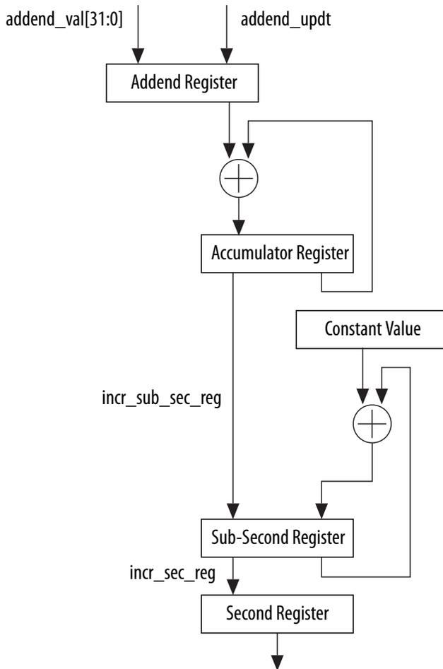
The System Time Update logic requires a 50-MHz clock frequency to achieve 20-ns accuracy. The frequency division ratio (FreqDivisionRatio) is the ratio of the reference clock frequency to the required clock frequency. Hence, if the reference clock (`clk_ptp_ref_i`) is for example, 66 MHz, this ratio is calculated as  $66 \text{ MHz} / 50 \text{ MHz} = 1.32$ . Hence, the default addend value to program in the register is  $232 / 1.32$ , `0xC1F07C1F`.
