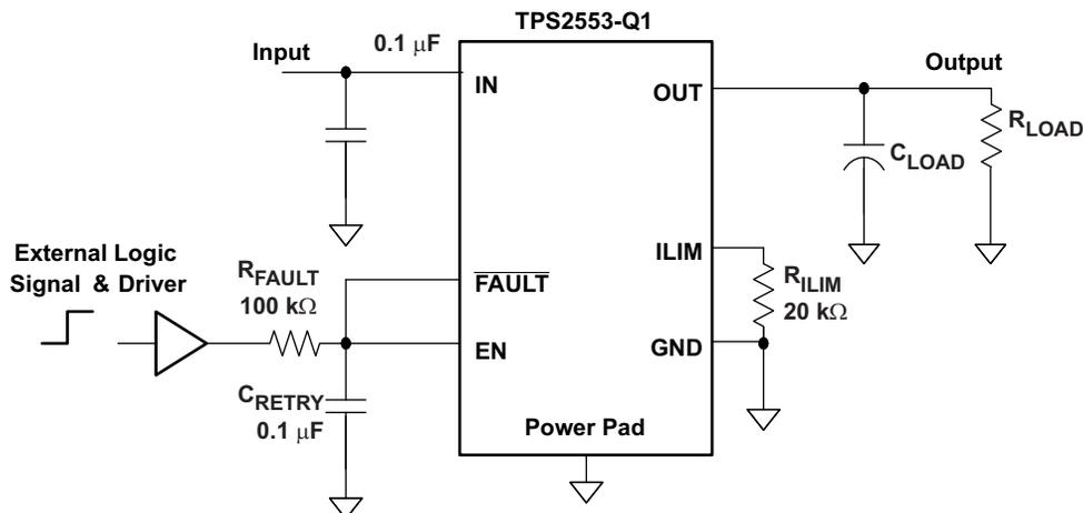
Figure 26. Auto-Retry Functionality With External EN Signal
