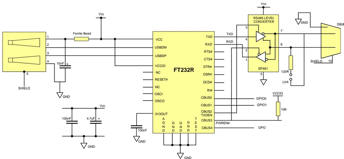
**Figure 7.2 Application Example Showing USB to RS485 Converter**
