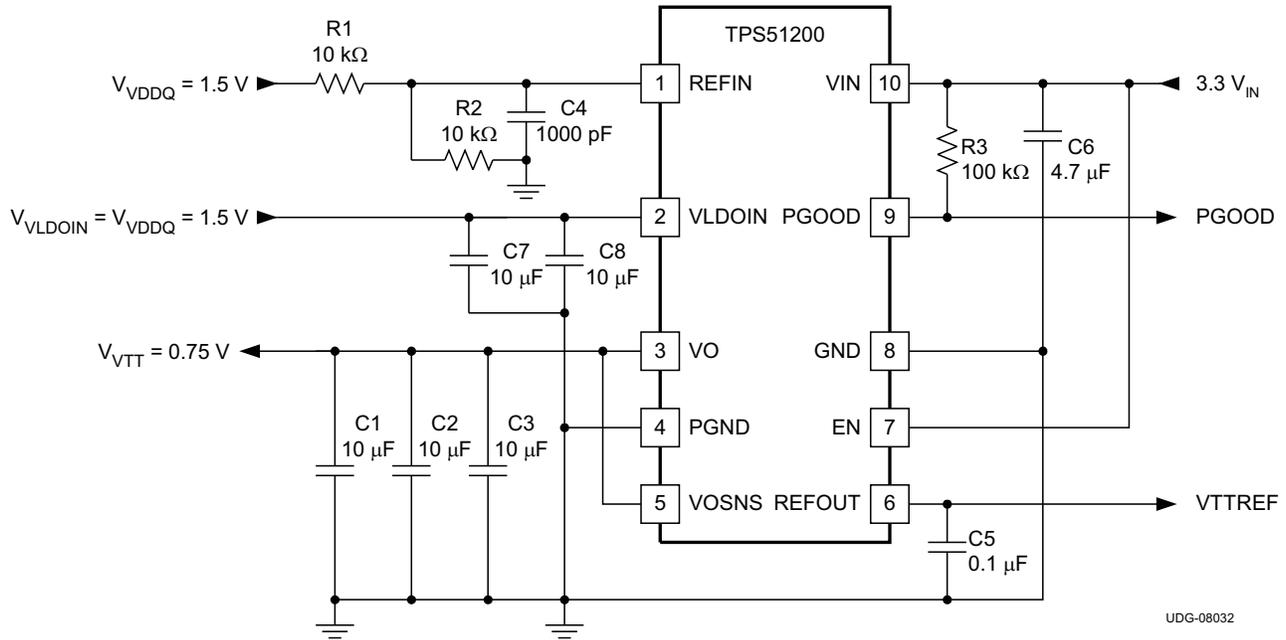
**Figure 29. 3.3-V<sub>IN</sub>, DDR3 Tracking Configuration**
