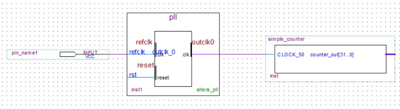
**Figure 3-18 Connecting the PLL symbol and Input port**
