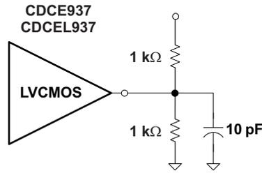
Figure 1. Test Load
