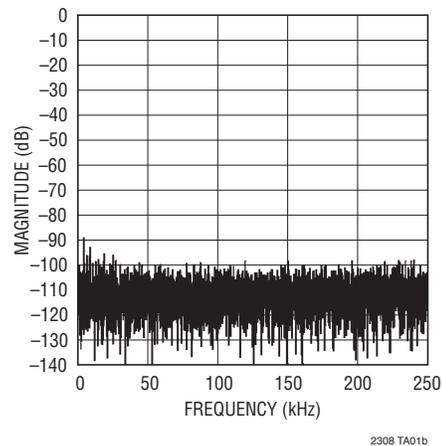
Figure 5. 1kHz Sine Wave 8192 Point FFT Plot
