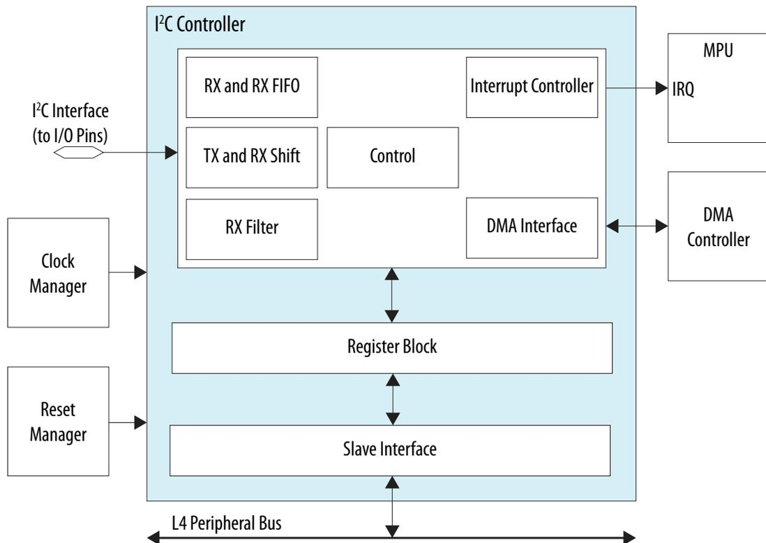
The I<sup>2</sup>C controller consists of the following modules and interfaces:
