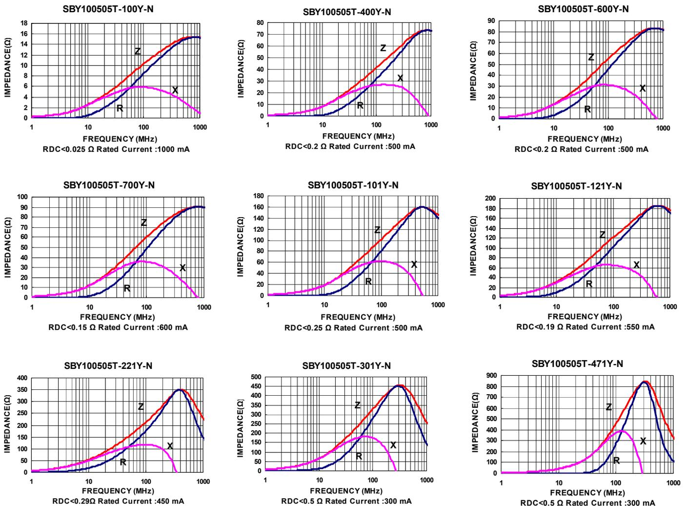
**Test Instruments :** Agilent E4991A Impedance / Material Analyzer
