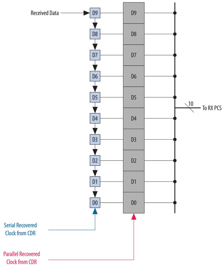
Figure 1-16: Deserializer Bit Order with 10-bit Deserialization Factor
