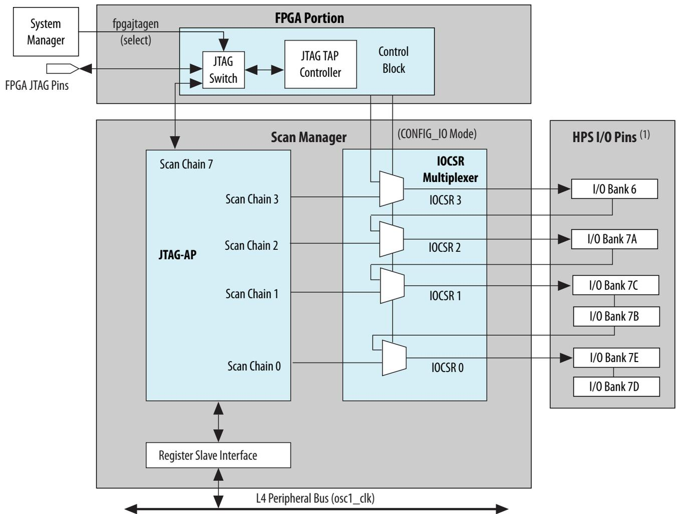
The processor accesses the scan manager through the register slave interface connected to the level 4 (L4) peripheral bus.
