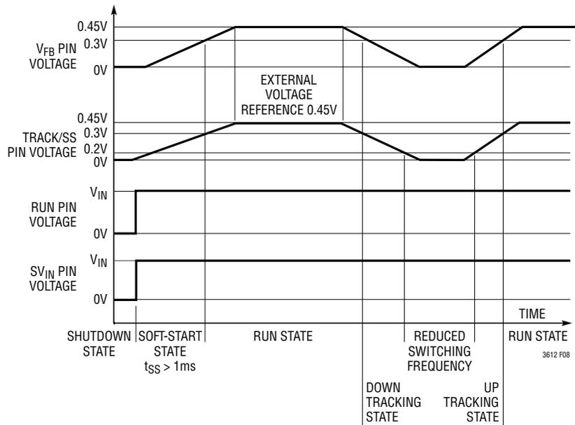
Figure 8. DDR Pin Tied to S<sub>VIN</sub>. Example DDR Application
