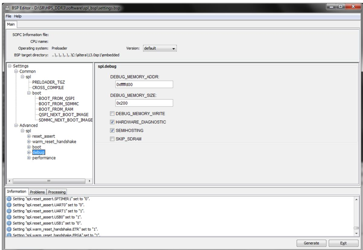
2. Enable semihosting in the debugger, by typing `set semihosting enabled true` at the command line in the debugger.
