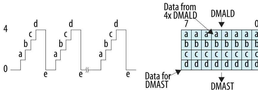
This example has a static requirement of zero MFIFO buffer entries and a dynamic requirement of four MFIFO buffer entries.
