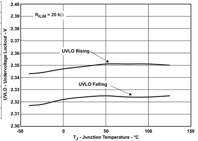
Figure 17. UVLO – Undervoltage Lockout - V
