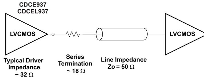
Figure 2. Test Load for 50-Ω Board Environment
