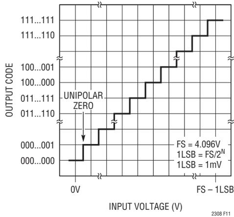
Figure 11. LTC2308 Unipolar Transfer Characteristics (Straight Binary)
