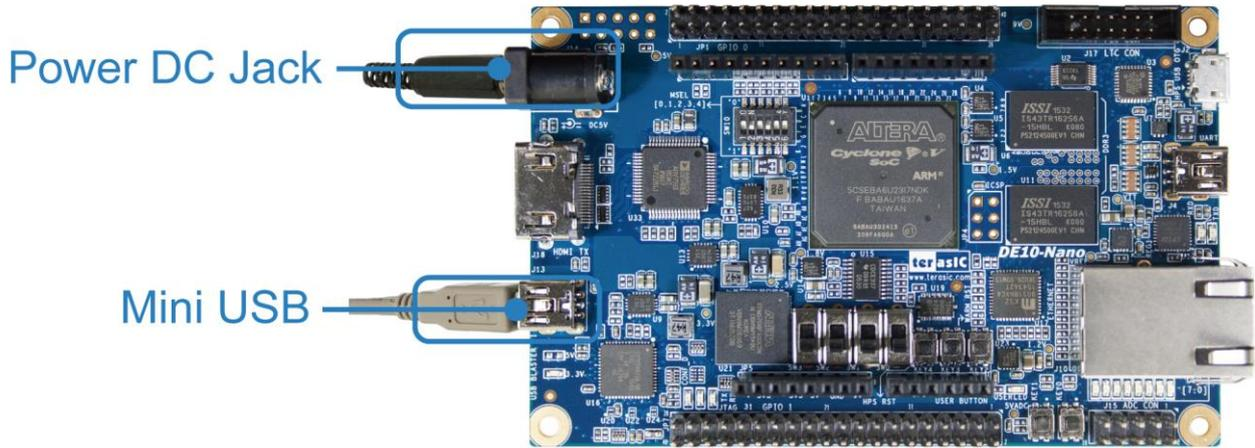
Figure 1-2 Connection Setup
