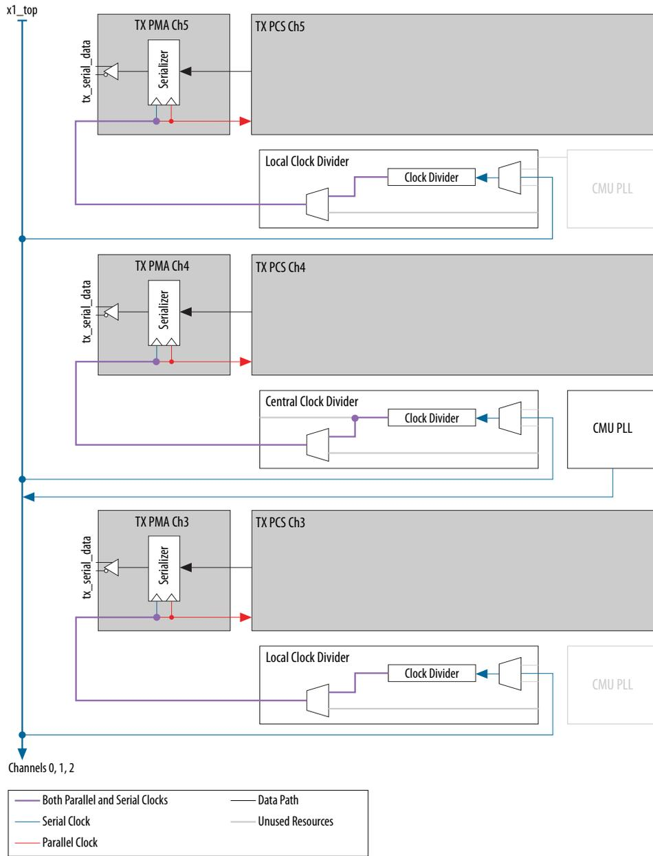
Figure 2-10: Three Non-Bonded Transmitter Channels Driven by CMU PLL using x6 and xN Clock Lines Across Multiple Transceiver Banks
