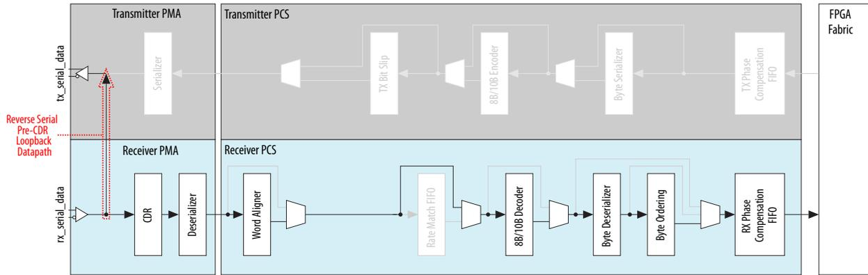
Note: Grayed-out blocks are not active when the reverse serial pre-CDR loopback is enabled.
