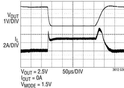
**Start-Up from Shutdown with Prebiased Output (Forced Continuous Mode)**
