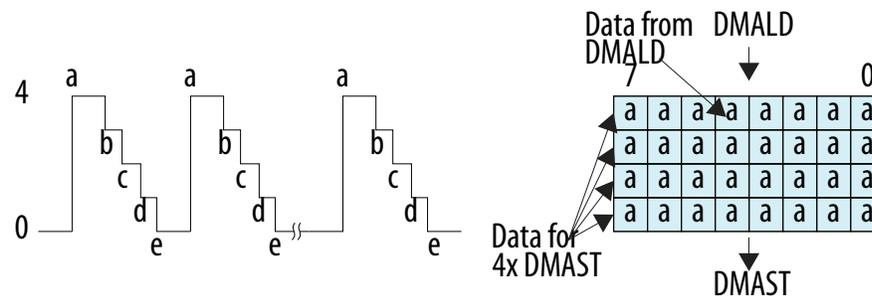
This example has a static requirement of zero MFIFO buffer entries and a dynamic requirement of four MFIFO buffer entries.
