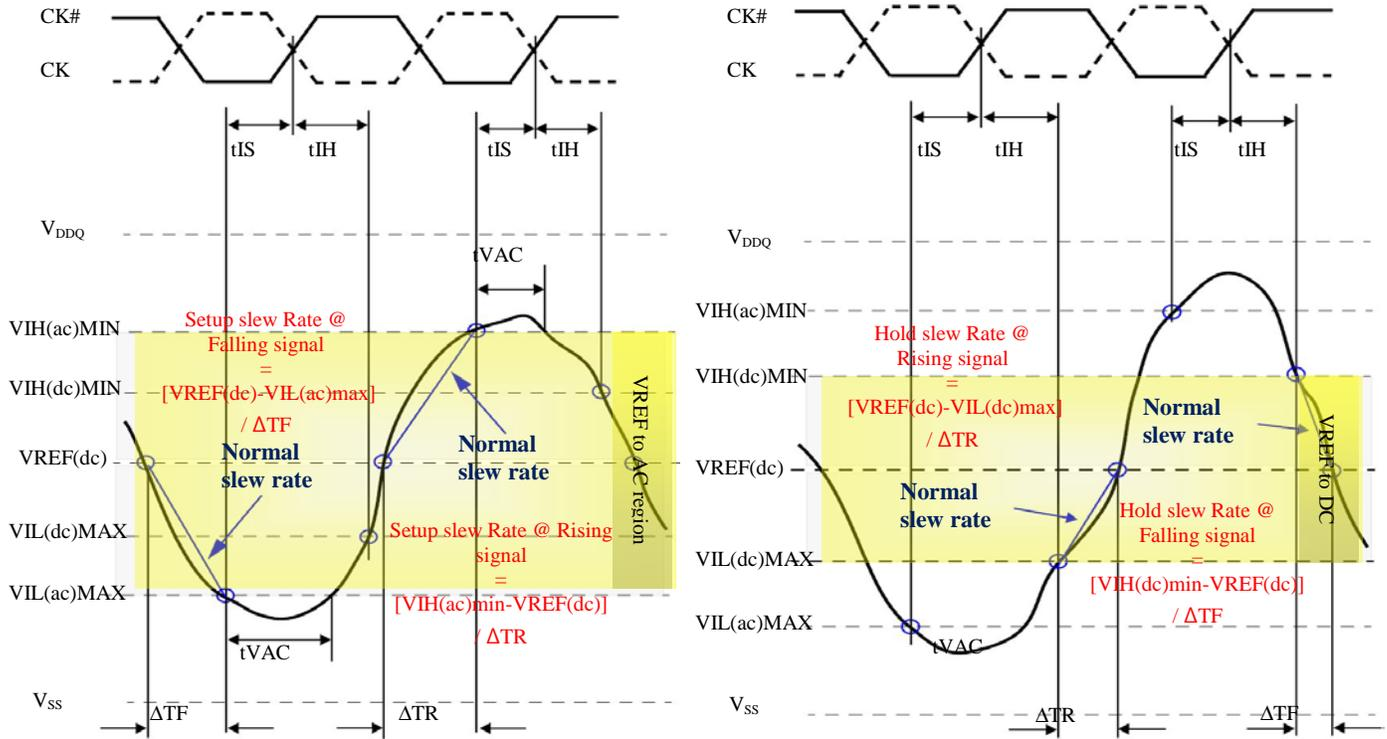
9.6.5.2 Tangent line for setup time tIS(left) and hold time tIH(right) - ADD/CMD with respect to clock
