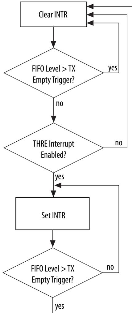
The threshold level is programmed into `FCR.TET`. The available empty thresholds are empty, 2,  $\frac{1}{4}$ , and  $\frac{1}{2}$ . The optimum threshold value depends on the system's ability to begin a new transmission sequence in a timely manner. However, one of these thresholds should prove optimum in increasing system performance by preventing the transmit FIFO buffer from running empty.
