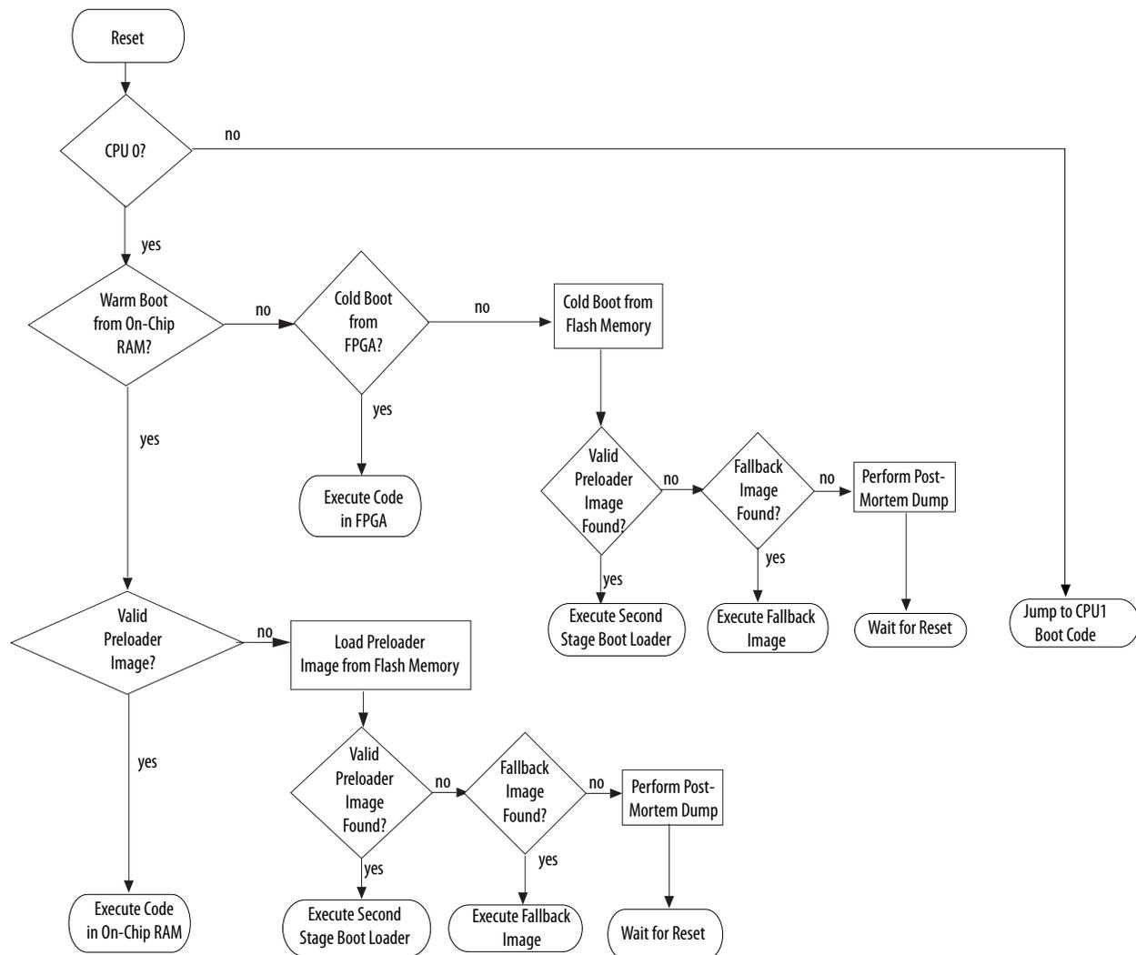
After a reset, the BootROM code determines which CPU it is executing on. If it is executing on CPU 1, then control is passed to CPU1 and the boot ROM execution is complete. This event only happens if the user code releases CPU1 without resetting the exception vectors.
