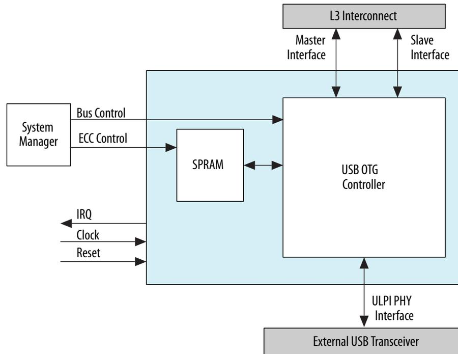
The USB OTG controller connects to the level 3 (L3) interconnect through a slave interface, allowing other masters to access the control and status registers (CSRs) in the controller. The controller also connects to the L3 interconnect through a master interface, allowing the DMA engine in the controller to move data between external memory and the controller.
