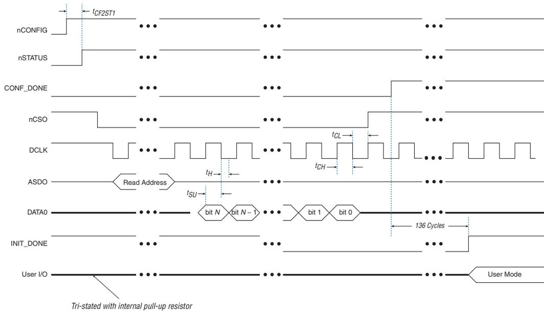
Table 14–25 shows the timing parameters for AS configuration mode.
