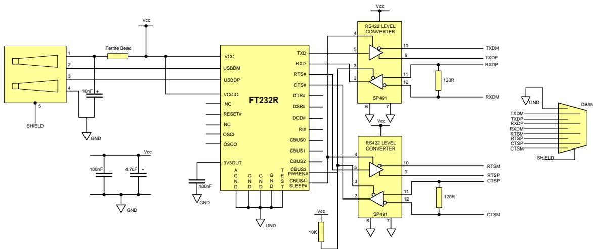
**Figure 7.3 USB to RS422 Converter Configuration**
