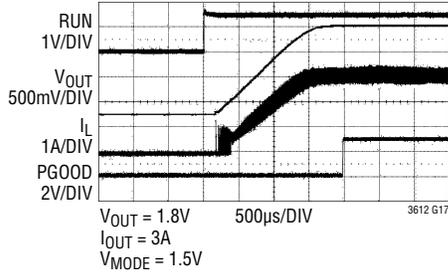
**Tracking Up/Down in Forced Continuous Mode, DDR Pin Tied to 0V**
