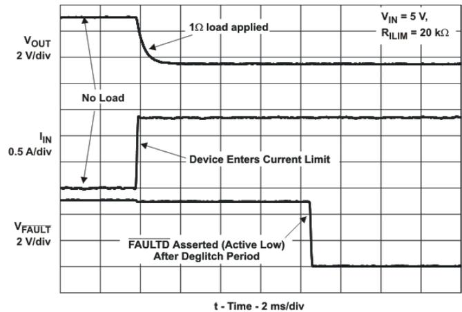
Figure 13. No Load to 1Ω Transient Response
