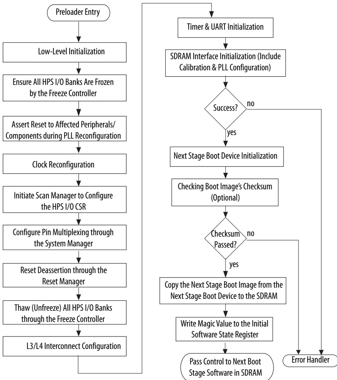
Low-level initialization steps include reconfiguring or disabling the L4 watchdog 0 timer, invalidating the instruction cache and branch predictor, remapping the on-chip RAM to the lowest memory region, and setting up the data area.
