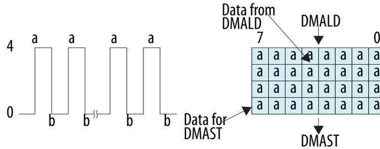
This example has a static requirement of zero MFIFO buffer entries and a dynamic requirement of four MFIFO buffer entries.
