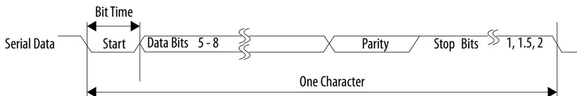
An additional parity bit may be added to the serial character. This bit appears after the last data bit and before the stop bit(s) in the character structure to provide the UART controller with the ability to perform simple error checking on the received data. †
