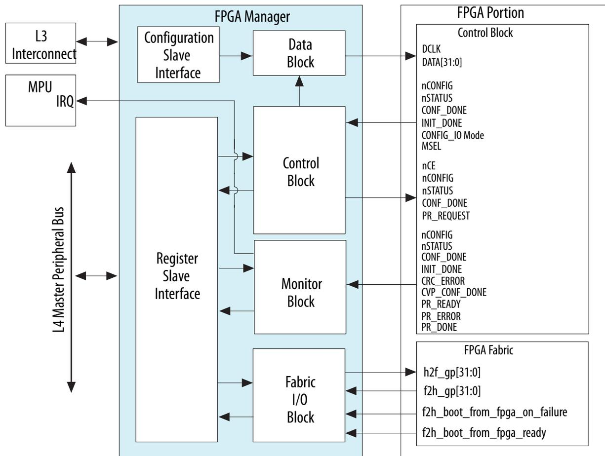
The register slave interface connects to the level 4 (L4) master peripheral bus for control and status register (CSR) access. The configuration slave interface connects to the level 3 (L3) interconnect for the microprocessor unit (MPU) subsystem or other masters to write the FPGA configuration image to the FPGA control block (CB) when configuring the FPGA portion of the SoC device.
