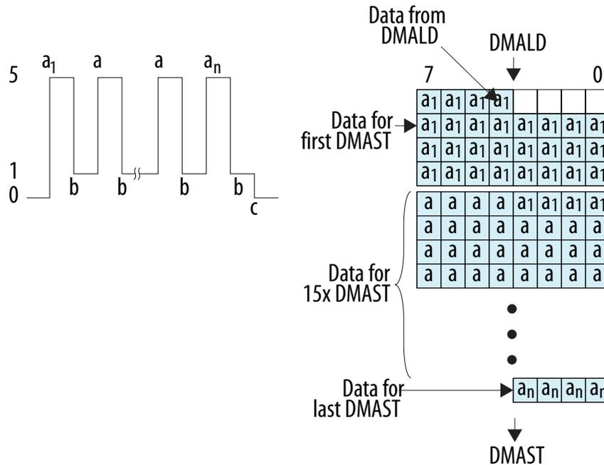
This example has a static requirement of one MFIFO buffer entry and a dynamic requirement of four MFIFO buffer entries.
