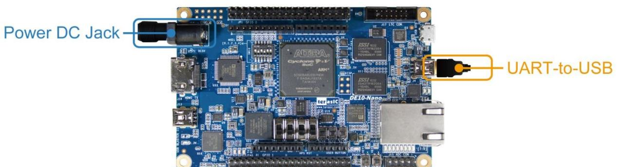
Figure 5-1 Hardware Setup for UART Terminal
