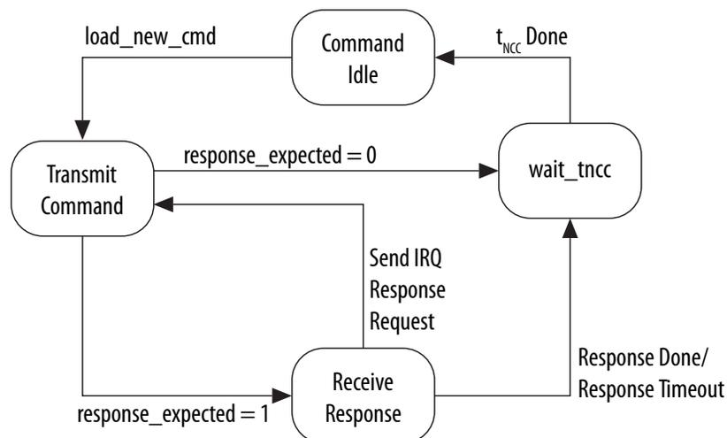
The command path state machine performs the following functions, according to `cmd` register bit values:<sup>†</sup>
