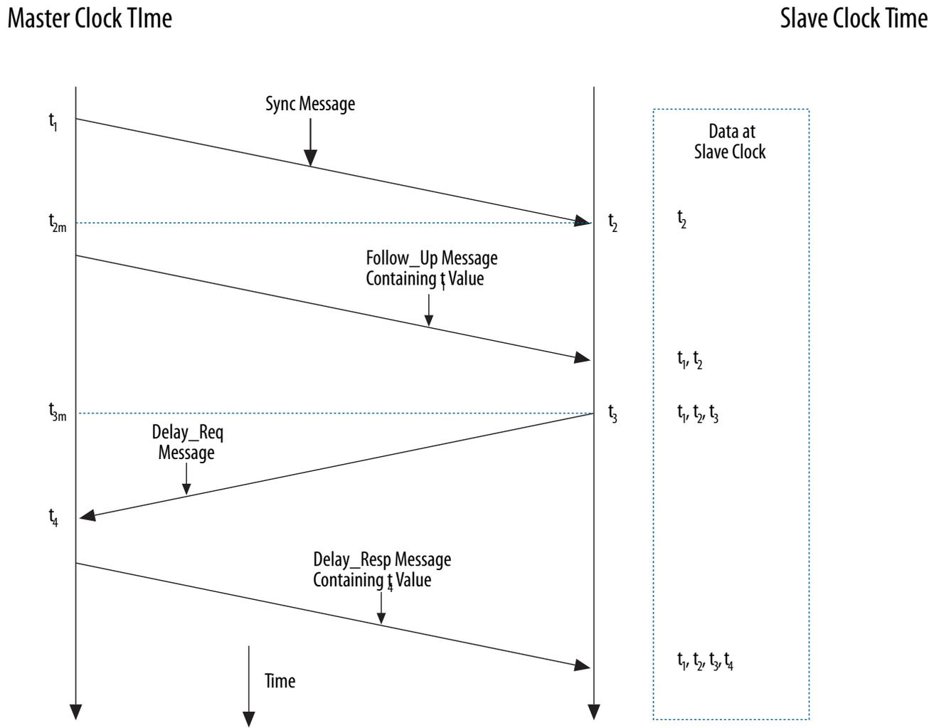
The PTP uses the following process for synchronizing a slave node to a master node by exchanging the PTP messages:
