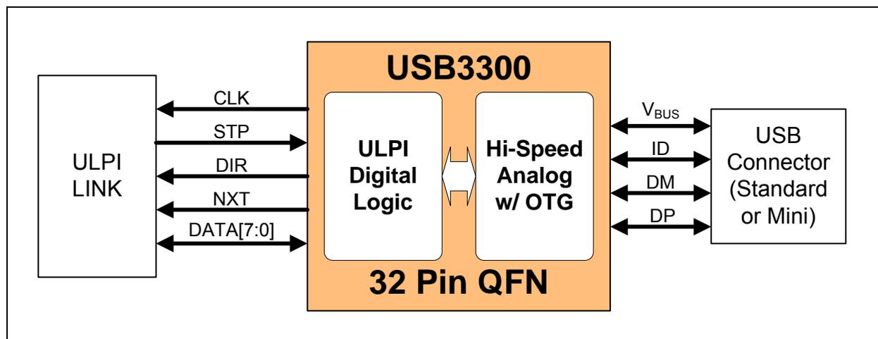
**Figure 1.1 Basic ULPI USB Device Block Diagram**
