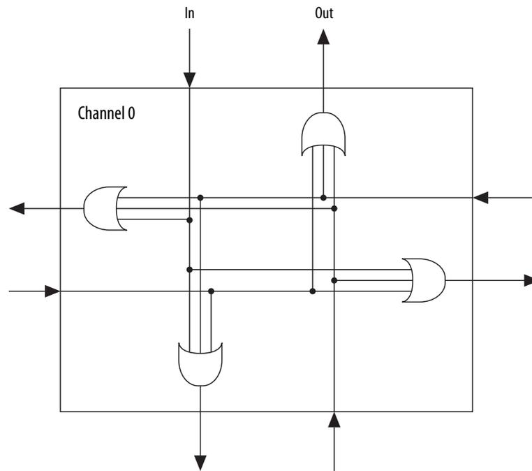
**Figure 10-5: CTI Trigger Connections**
