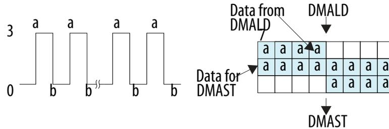
In this example, the destination address is not 64-bit aligned, it requires three rather than the expected two MFIFO buffer entries.
