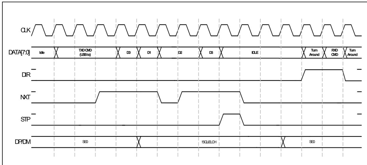
**Figure 6.6 ULPI Transmit**
