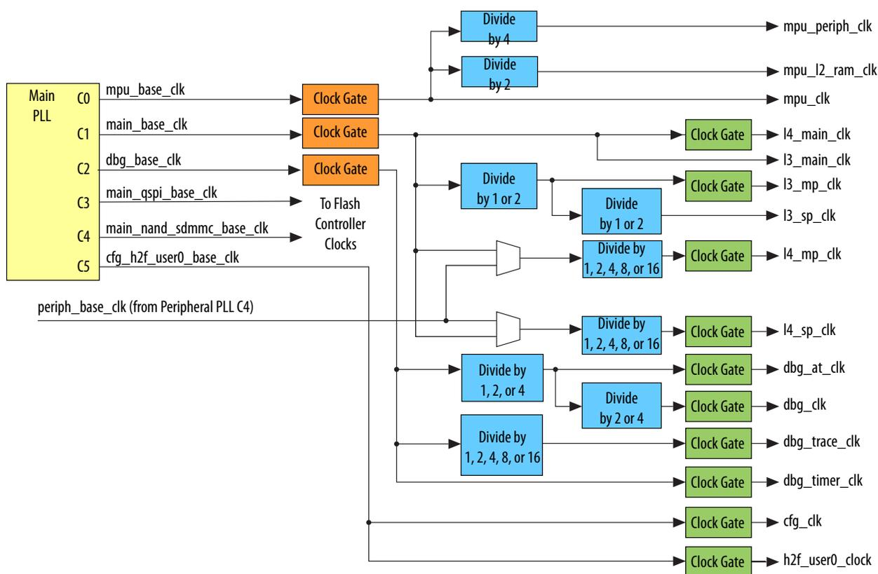
The clocks derived from main PLL C0-C2 outputs are hardware-managed, meaning hardware ensures that a clean transition occurs, and can have the following control values changed dynamically by software write accesses to the control registers:
