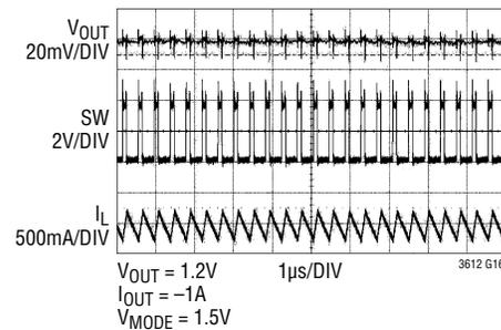
**TYPICAL PERFORMANCE CHARACTERISTICS**  $V_{IN} = 3.3V$ ,  $RT/SYNC = SV_{IN}$ , unless otherwise noted.
