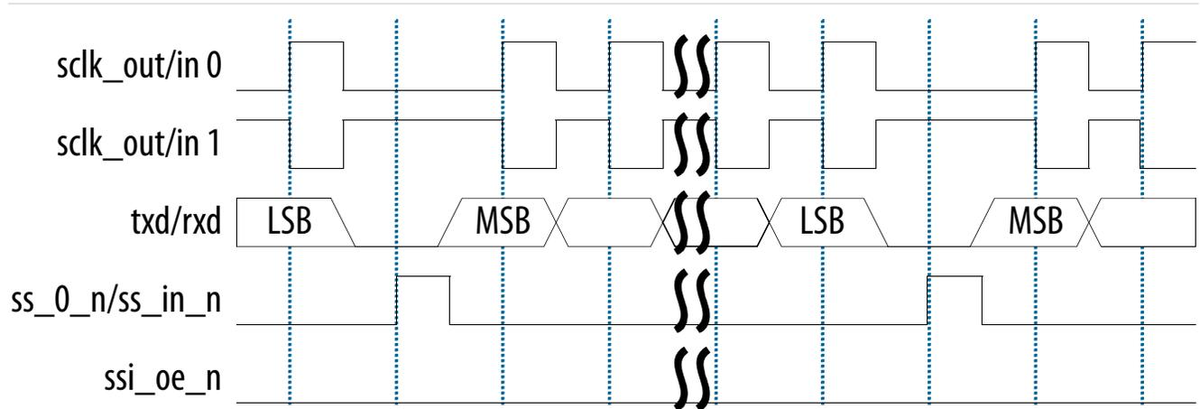
Figure 19-8: Serial Format Continuous Transfers ( $SCPH = 1$ )
