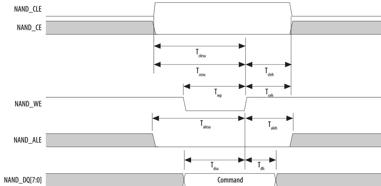
Figure 15: NAND Address Latch Timing Diagram
