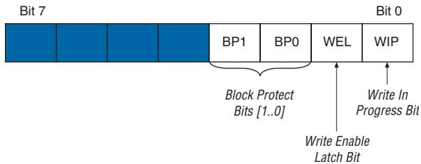
Setting the write in progress bit to 1 indicates that the serial configuration device is busy with a write or erase cycle. Resetting the write in progress bit to 0 means no write or erase cycle is in progress.
