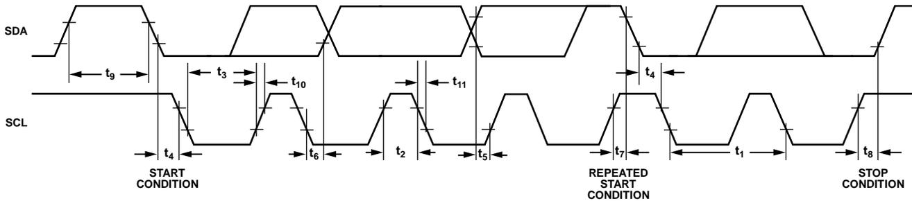
Figure 41. I<sup>2</sup>C Timing Diagram
