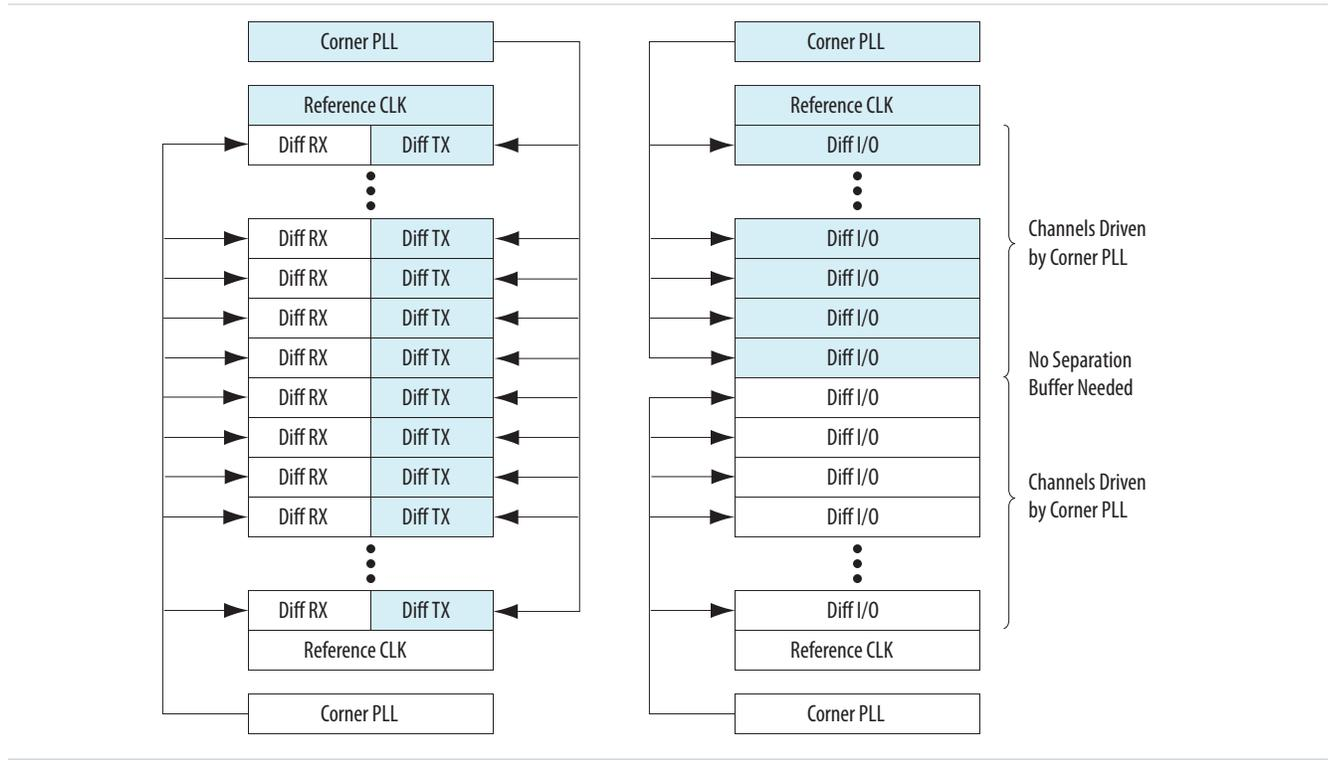
**Figure 5-3: Invalid Placement of Differential I/Os Due to Interleaving of Channels Driven by the Corner PLLs**
