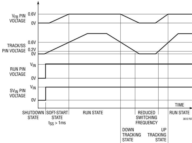
Figure 7. DDR Pin Not Tied to S<sub>VIN</sub>
