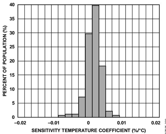
Figure 20. Y-Axis Sensitivity Temperature Coefficient,  $V_S = 2.5 V$
