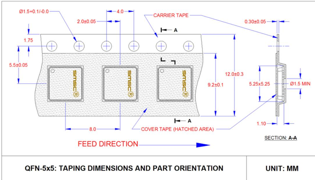
Figure 8.1 QFN, 5x5 Taping Dimensions and Part Orientation
