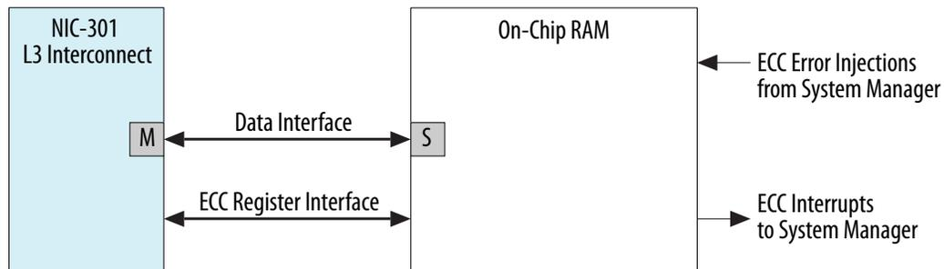
**Note:** You must initialize the on-chip RAM before you enable the ECC support to prevent false ECC interrupts triggered by uninitialized bits.
