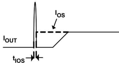
Figure 3. Response Time to Short Circuit Waveform
