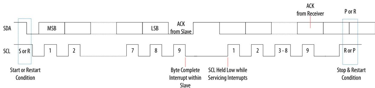
The I<sup>2</sup>C controller is a synchronous serial interface. The SDA line is a bidirectional signal and changes only while the SCL line is low, except for STOP, START, and RESTART conditions. The output drivers are open-drain or open-collector to perform wire-AND functions on the bus. The maximum number of devices on the bus is limited by only the maximum capacitance specification of 400 pF. Data is transmitted in byte packages. †
