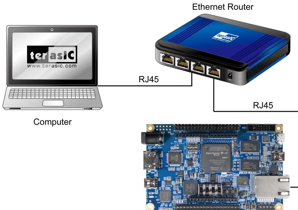
**Figure 3-1 Ethernet Setup**
