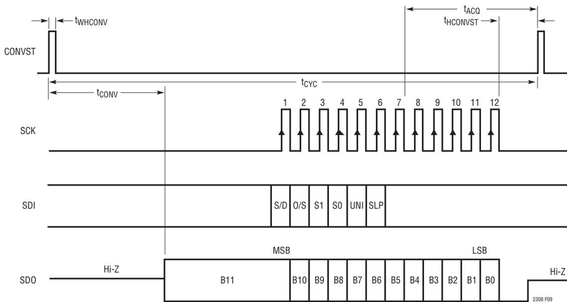
Figure 9. LTC2308 Timing with a Short CONVST Pulse
